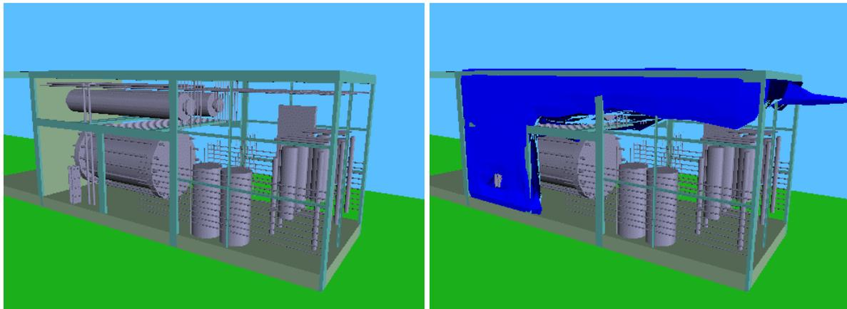
Figure 4. Visualisation of the gas dispersion model of the hydrogen production container (without cladding). Left: Before leakage. Right: Extents of lower flammability limit for hydrogen/air mixture inside container after 60 seconds.
