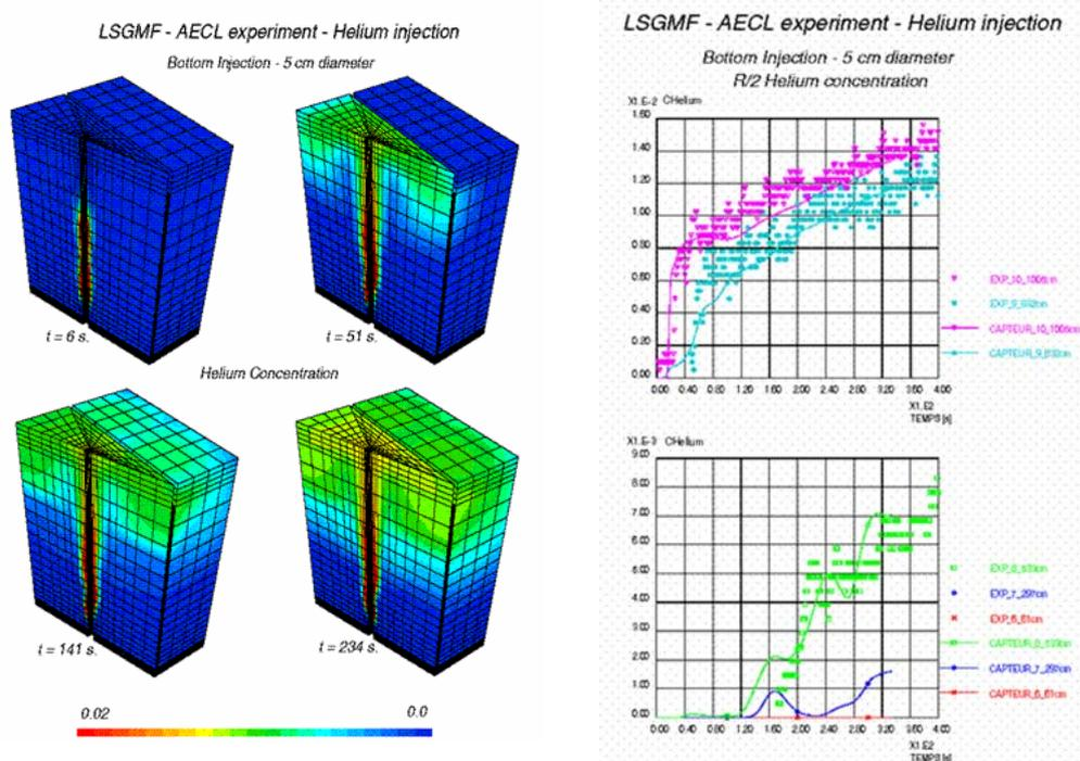
Figure 4: CAST3M simulations: on the left, Helium concentration isolines as different times, and on the right, comparison between computed results and experimental data
