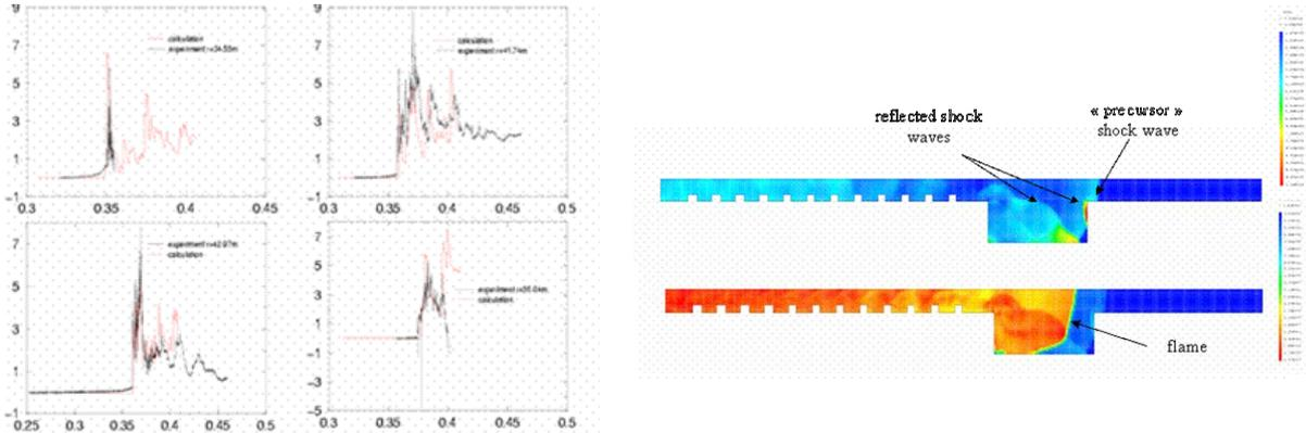
Figure 15: STH06 Fast deflagration calculation: on the left, comparison between predicted values and experimental measurements, on the right, pressure and temperature isolines (from [16])
