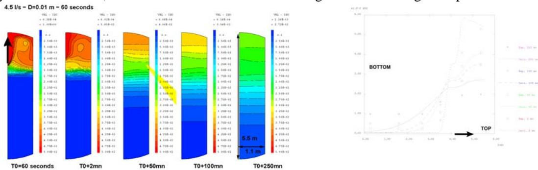
Figure 1: (left) H<sub>2</sub> concentration isolines at different times, showing a diffusion-dominated mixing process once the injection is stopped; (right) Comparison between predicted and measured values.
