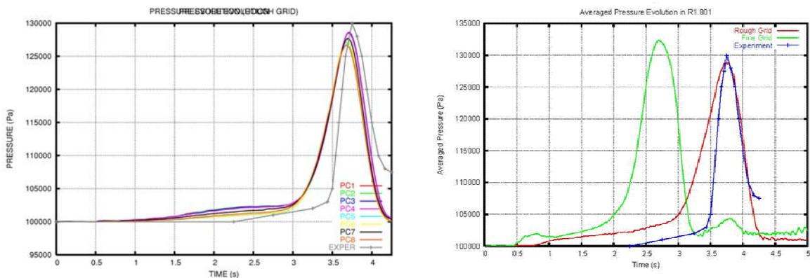
Figure 10: Computed pressure vs. data. Left, coarse mesh results. Right, effect of grid refinement
