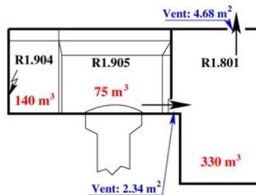
Figure 8: HDR test E12.3.2. Sketch of the problem.
