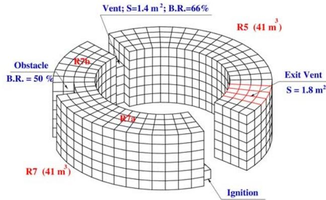
Figure 12: BMC test Ex29. Geometry
