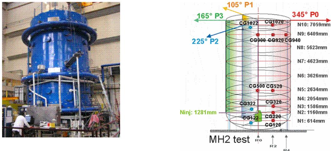
Figure 5: View of the MISTRA facility and position of sensors for the MH1 (and MH2) tests
