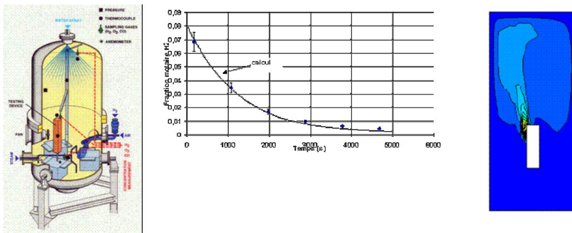
Figure 17: From left to right, diagram of the KALI facility of CEA, numerical predictions vs. experimental measurements of global hydrogen concentration as a function of time, and temperature contours showing the thermal plume exiting from the recombiner outlet.
