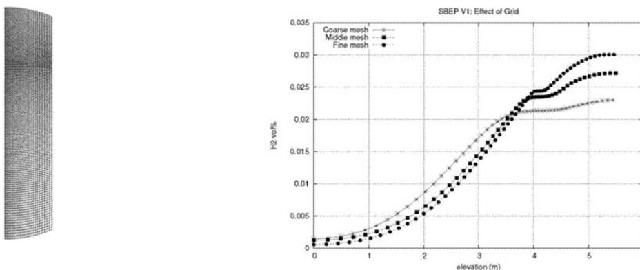
Figure 2: Example of grid used (Medium grid of 7400 nodes), and grid sensitivity analysis of the results, based on a series of grids with a refinement factor of 2 in each direction.
