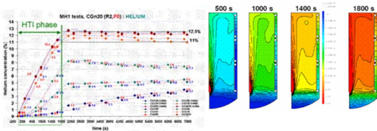
Figure 6: (left) Measured concentrations in the different sensor locations as a function of time; (right) Predicted He concentration contours at different times during the injection;
