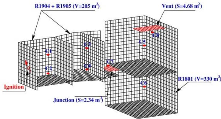
Figure 9: Geometry of the problem with probes positioning.
