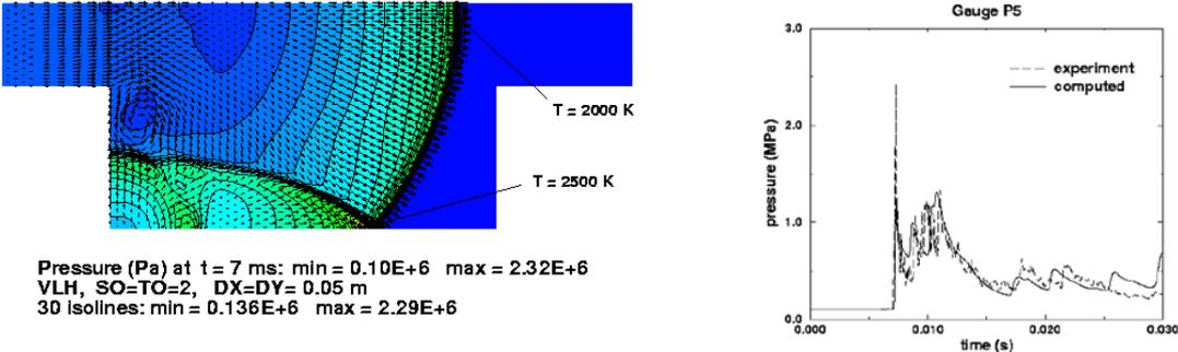
Figure 16: On the left, pressure isolines from the CAST3M two-dimensional plane calculation, and on the right, comparison between computed results and pressure measurements.
