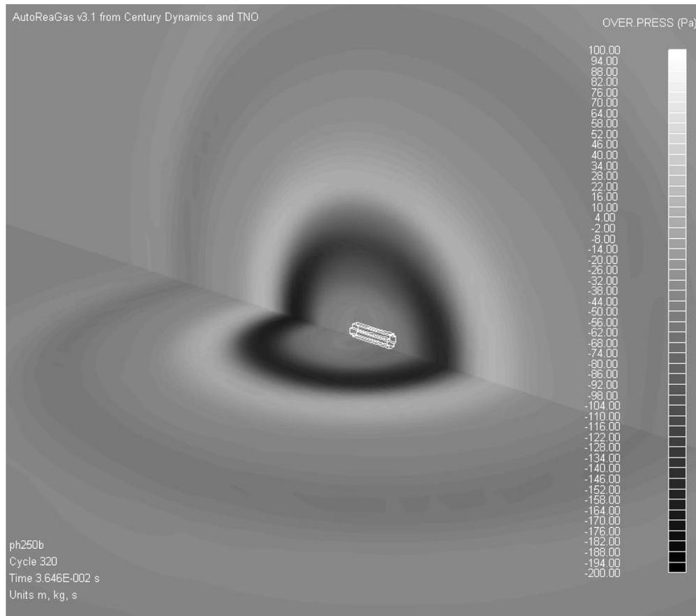
Figure 4. Overpressure generated by the ignition of the flammable cloud from a 250 m/sec outflow from a 6mm PRD device of a cylinder as a function of distance.
