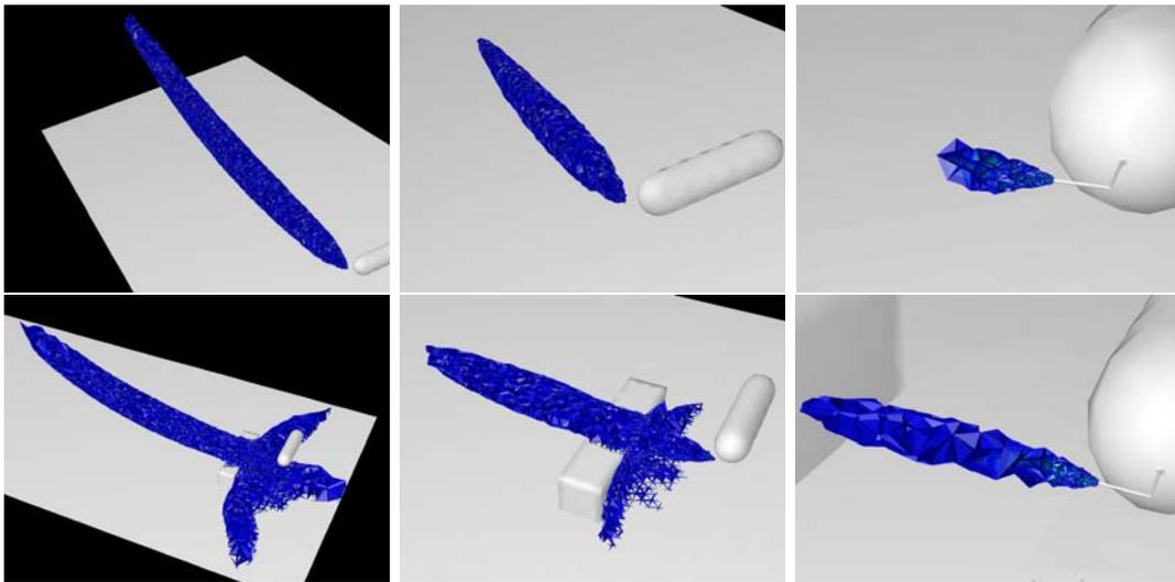
Figure 3. Molar fraction contours arising from a critical flow from a cylinder in the absence (top) and presence (bottom) of a wall. From left to right, the molar fractions are 2%, 4% and 15%.
