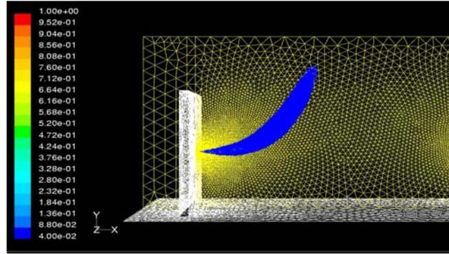
Figure 1. Simulation results 30 seconds after the leak began for the horizontal hydrogen jet. The mesh in the symmetry plane is also shown.
