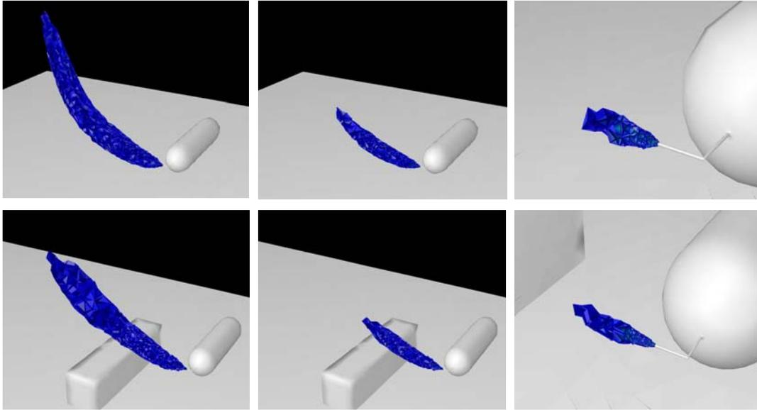
Figure 2. Molar fraction contours arising from a 250 m/sec leak from the pressure relief device of a pressurized cylinder in the absence (top) and presence (bottom) of a wall. From left to right, the molar fractions are 2%, 4% and 15%.
