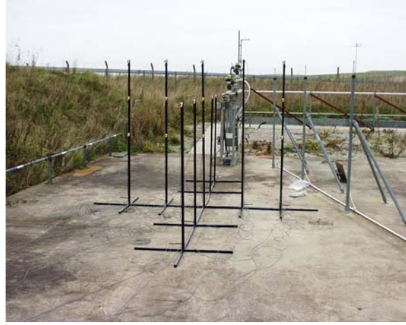
Figure 1(b). Oxygen depletion sensors for low pressure releases (towards the release nozzle)
