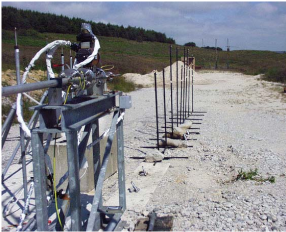
Figure 2(a). Oxygen depletion sensors for high pressure releases (behind release nozzle)
