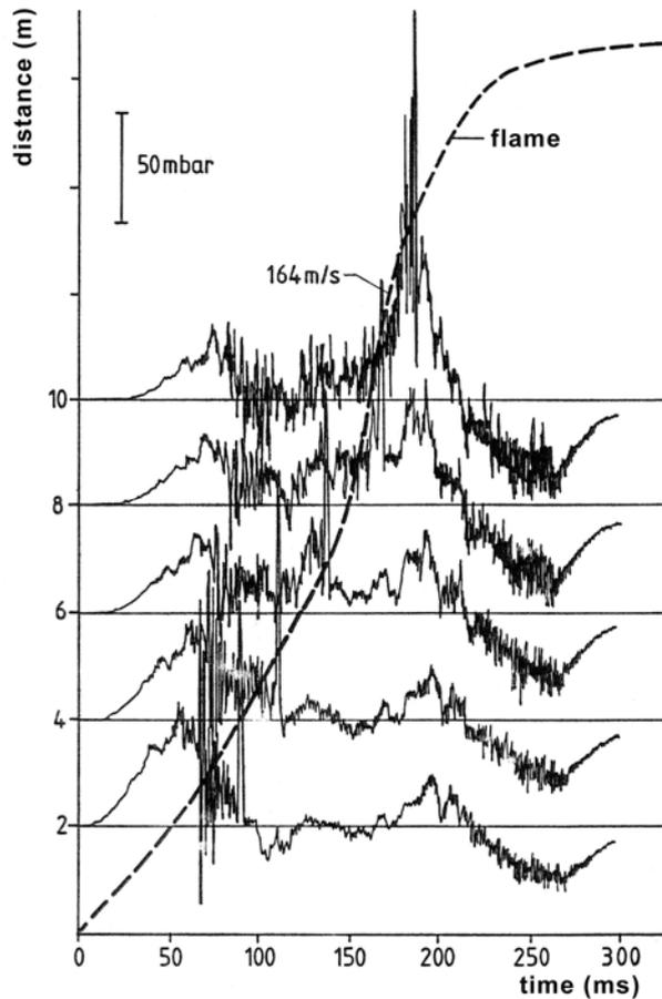
Figure 1. Flame propagation and pressure time histories for a quiescent hydrogen air mixture (37% H<sub>2</sub>) in a lane
