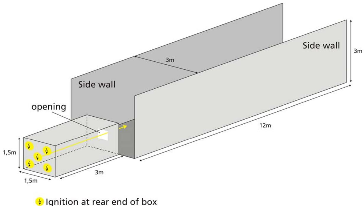
Figure 4. Test set up for the ignition of a hydrogen air mixture within a lane with a flame jet
