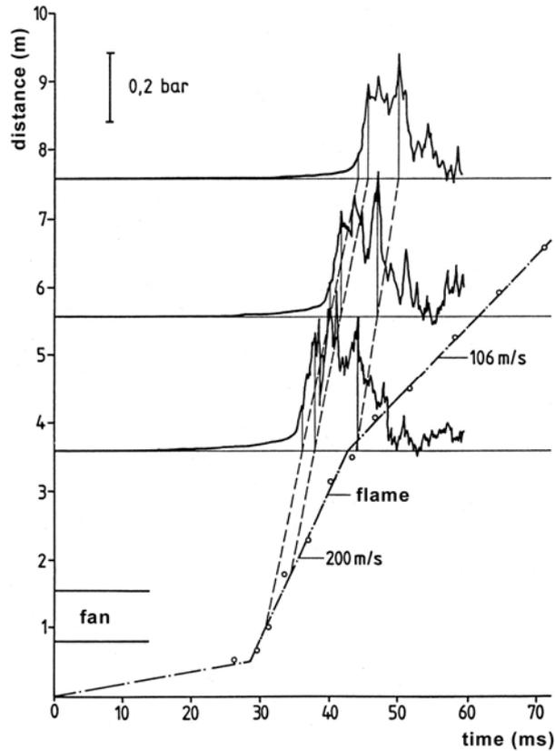
Figure 2. Flame propagation and pressure time histories for a turbulent hydrogen air mixture (41% H<sub>2</sub>) in a lane
