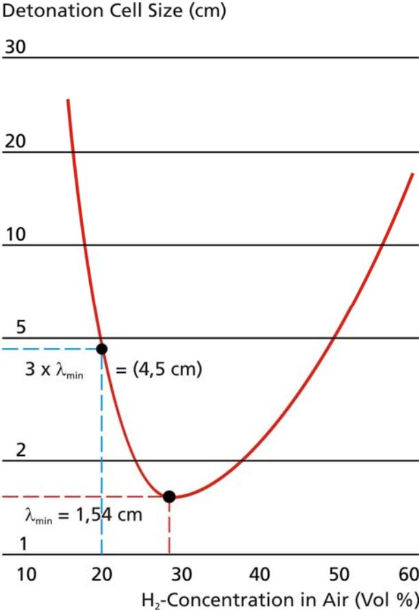
Figure 5. Scaling of DDT experiments with detonation cell  $\lambda$
