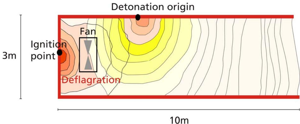
Figure 3. Propagation of flame front and detonation front in DDT experiment in a lane (turbulent hydrogen air mixture with 37% H<sub>2</sub>)
