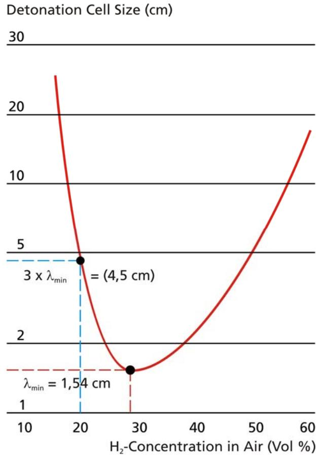
Figure 5. Scaling of DDT experiments with detonation cell  $\lambda$
