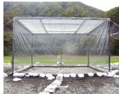
Figure 5. Experimental setup for explosion test with 200 m^3 tent
