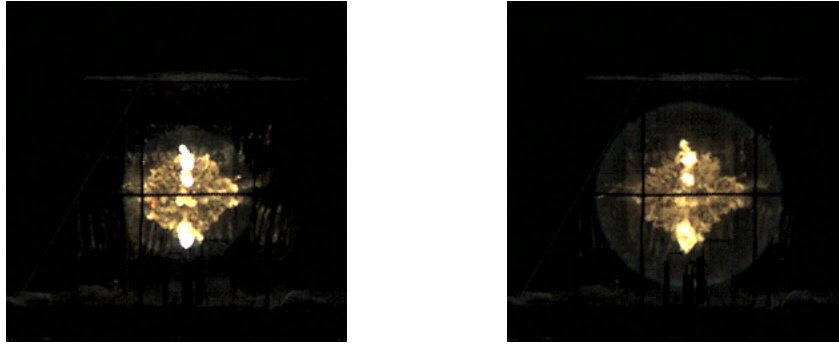
Figure 4. Typical results of high-speed photography obtained during the explosion test with 52.9 vol. % hydrogen/air mixture; initiated by a 0.1 kg booster of C-4 explosive. The photographs were respectively taken at 428 \mu s (left) and 628 \mu s (right) after initiation.
