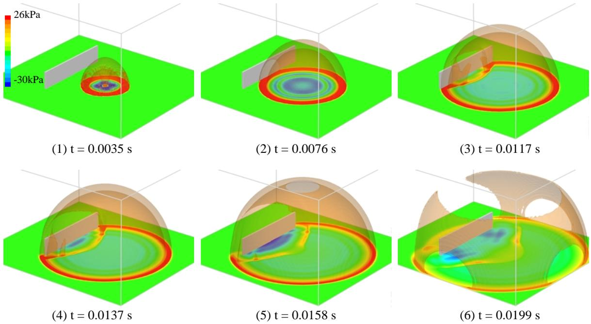
Figure 11. Instantaneous pressure contours and pressure iso-surfaces at various time steps in the detonation case (Case2)
