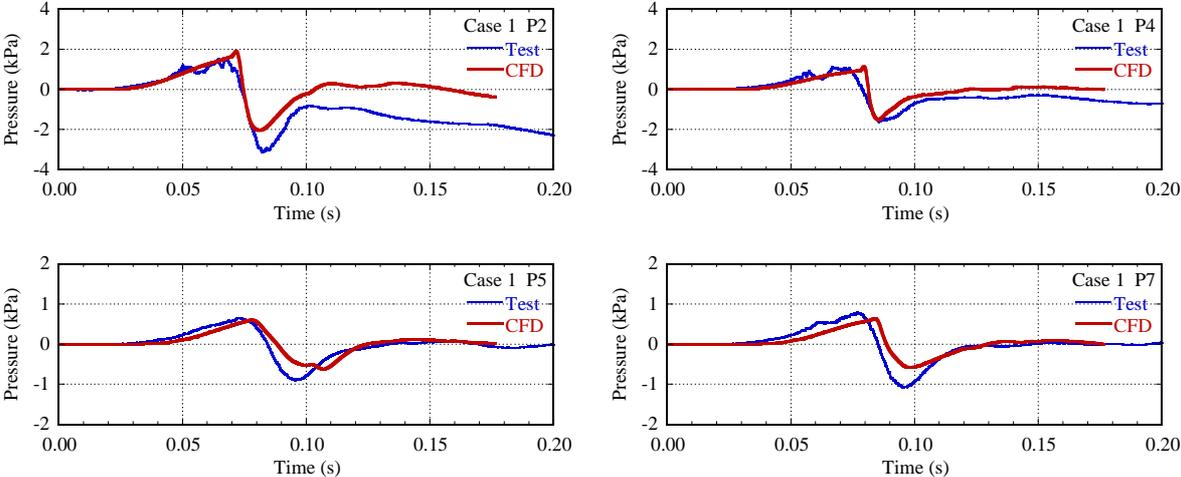
Figure 12. Blast pressure time histories on the barrier wall in Case1
