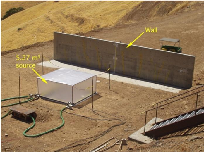
Figure 1. Wall and explosive source
