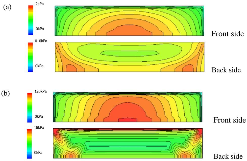
Figure 14. Distribution of the peak blast pressure on the barrier wall for (a) Case1 (b) Case2
