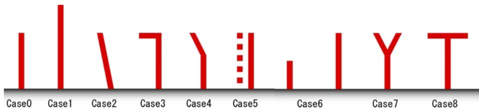
Figure 19. Analysed cross-sections of barrier wall shapes
