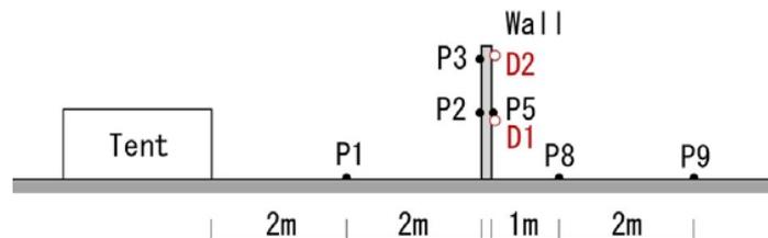
Figure 3. Pressure and displacement sensor locations along the ground surface
