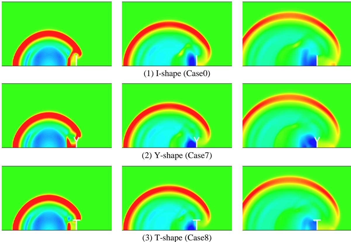
Figure 22. Instantaneous pressure contours in Case 0, Case 7 and Case 8
