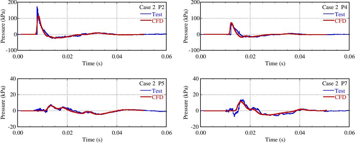
Figure 13. Blast pressure time histories on the barrier wall in Case2
