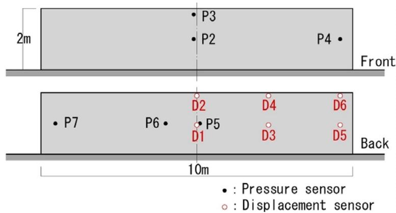
Figure 2. Pressure and displacement sensor locations on the surface of the wall
