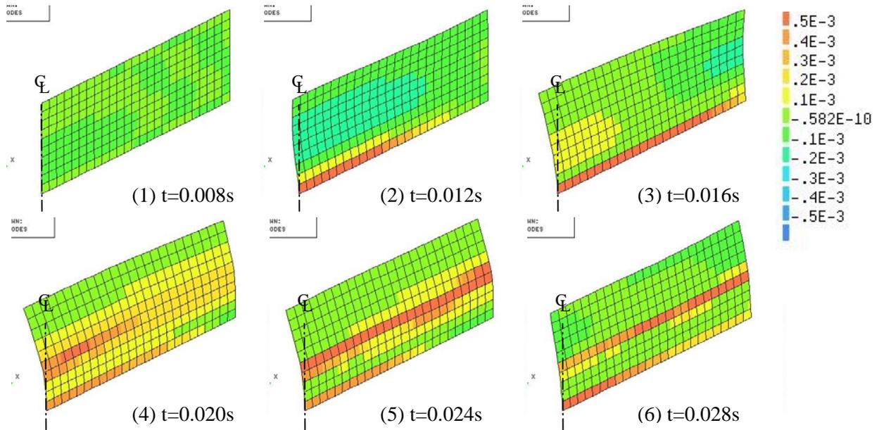
Figure 18. Concrete strains on the front surface of the wall in Case2 at various time steps
