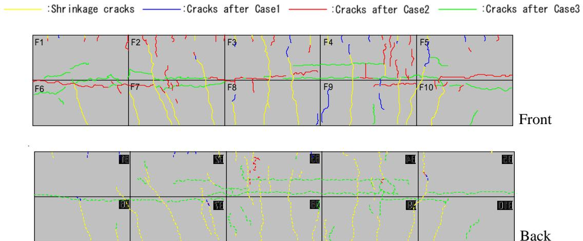
Figure 9. Distribution of cracks after each test
