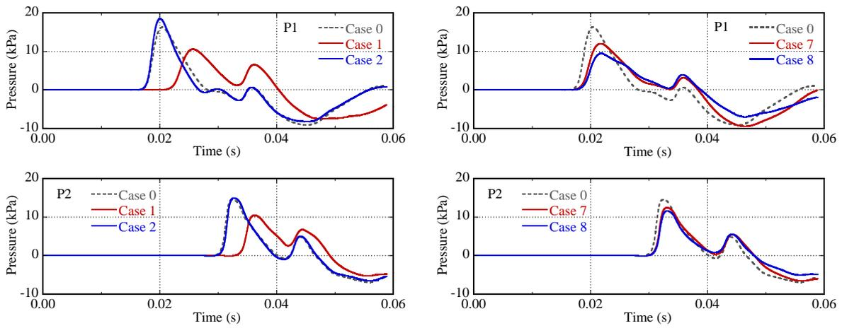
Figure 21. Blast pressure time histories at points P1 and P2
