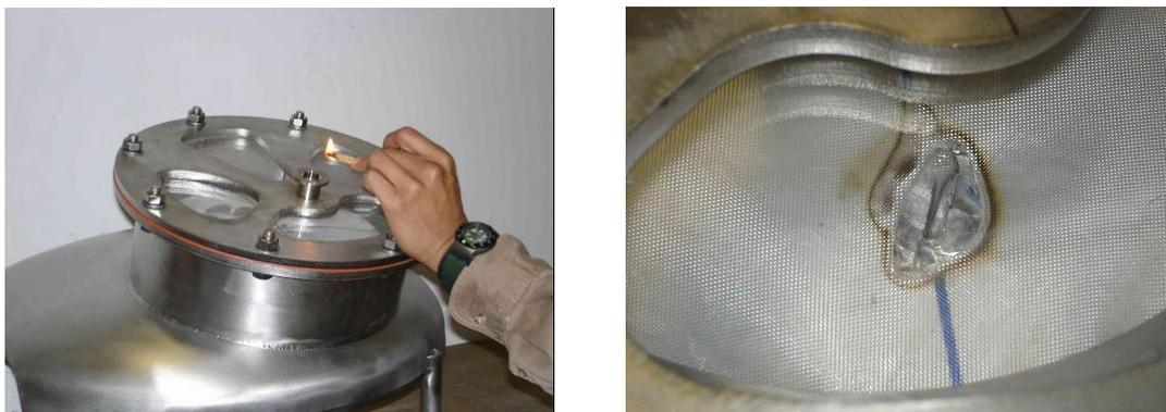
Figure 4: Multi layer insulation ignition test with pure oxygen atmosphere
