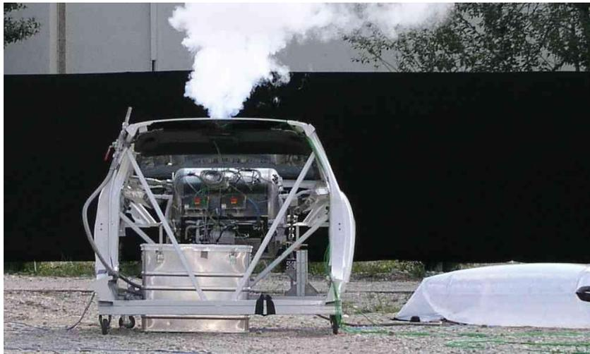
Figure 10: Investigation of pressure relief devices in case of vacuum loss (Source: ET GmbH.)
