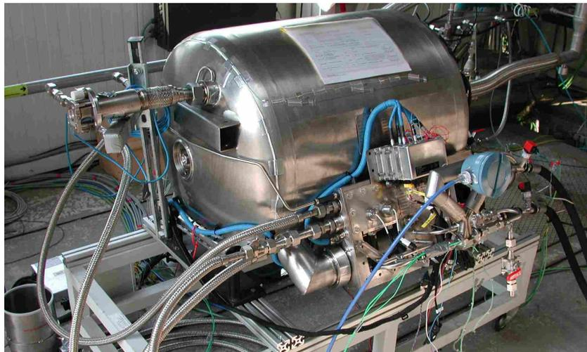
Figure 7: Functional test on the liquid hydrogen test bench (Source: ET GmbH.)
