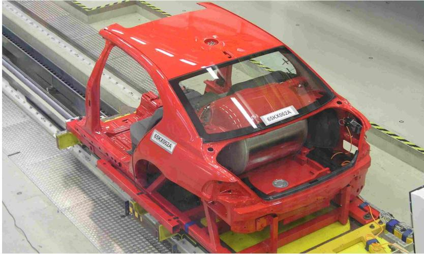
Figure 9: Skid test on the sliding test bench (Source: BMW Group)
