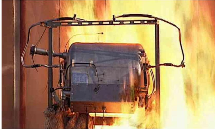
Figure 11: Bonfire test of a liquid hydrogen fuel tank (Source: BAM)
