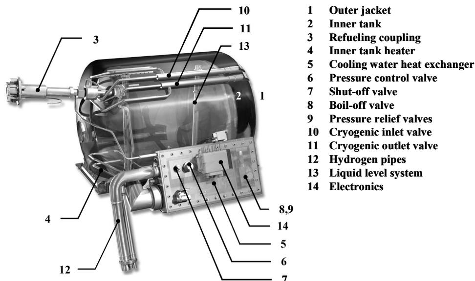
Figure 1: Liquid hydrogen fuel tank
