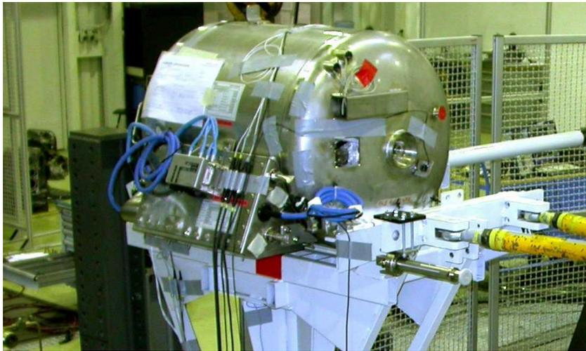
Figure 8: Dynamic vibration test of a liquid hydrogen fuel tank (Source: Magna Steyr)
