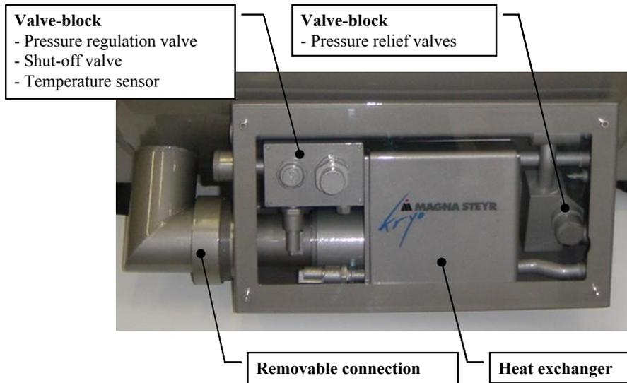
Figure 3: Auxiliary system box of a liquid hydrogen fuel tank
