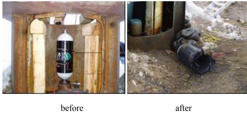
Figure 3. Cylinder situation (T-2: Type-3a, Axial, Disp. 88 mm, 35 MPa).
