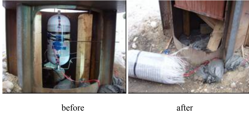
Figure 9. Cylinder situation (T-12: Type-3b, Axial, Disp. 100 mm, 35 MPa).
