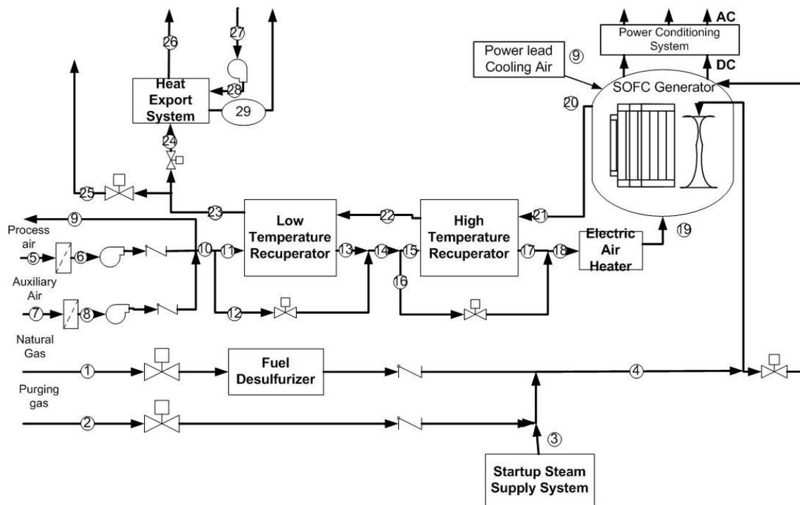
Figure 3. Simplified scheme of the CHP 100 SOFC Field Unit and the HES.
