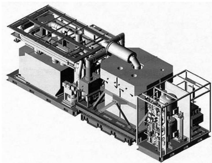
Figure 2. View of the SOFC field unit. (Courtesy of Siemens Westinghouse Power Corporation).
