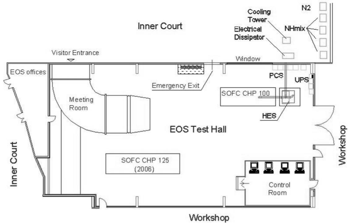
Figure 4. Lay-out of the EOS test hall.
