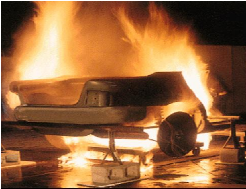
Figure 3. ECE R-34 Bonfire Test
