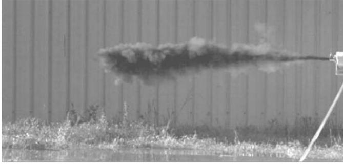
Figure 3: Powder expulsion cloud without external source of ignition
