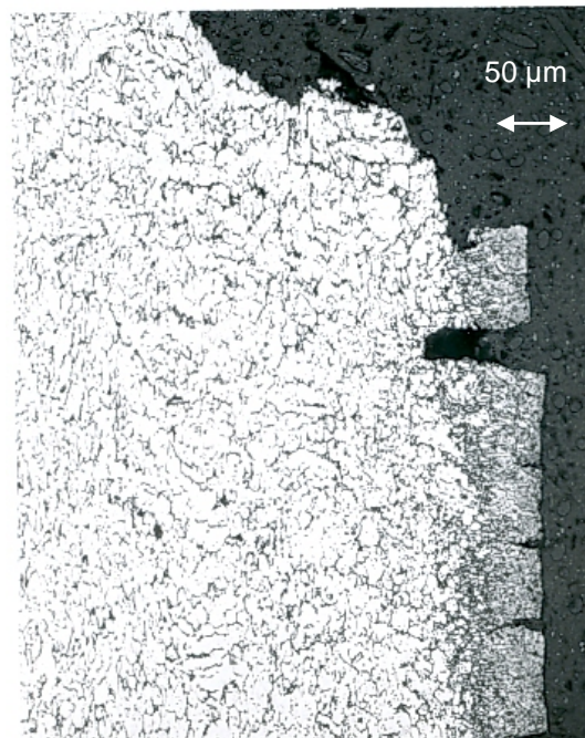
Figure 4. Hydride layer and secondary cracks on lateral surface of Ti Gr-12 specimen tested at a strain rate of 2 \times 10^{-7} \text{ s}^{-1} in sea water with a cathodic polarization of -1500 mV (Ag/AgCl).
