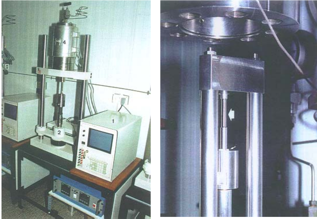
Figure 2. General view of the SSRT equipment. Detail of testing specimen in the autoclave.
