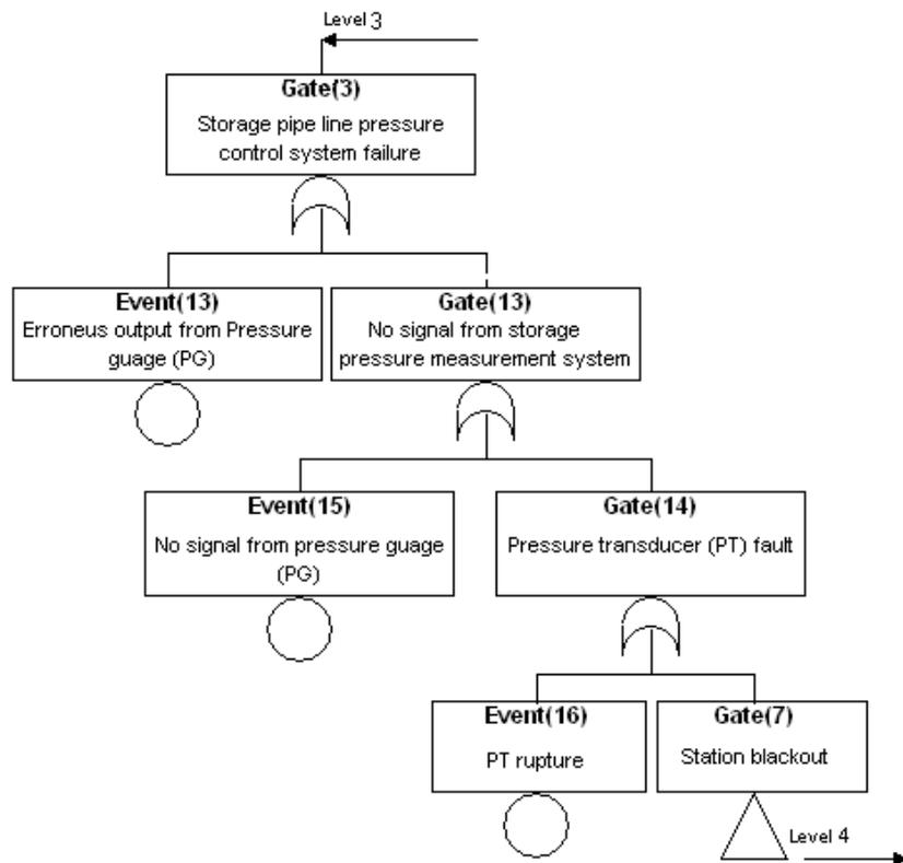
Figure 5. Storage pipeline pressure control system failure sub – fault tree.
