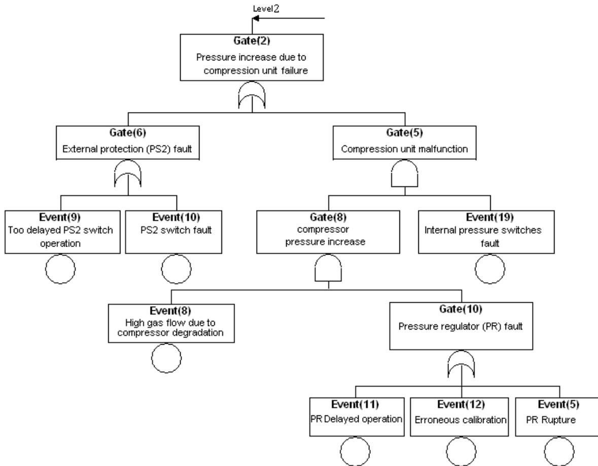
Figure 4. Pressure increase due to compression unit failure sub – fault tree.
