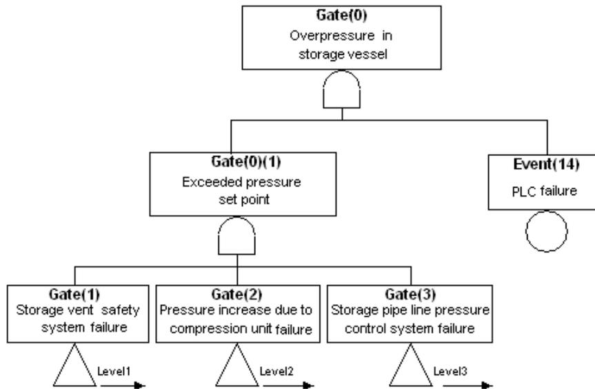
Figure 2. Storage vessel overpressure Top Event undeveloped fault tree.
