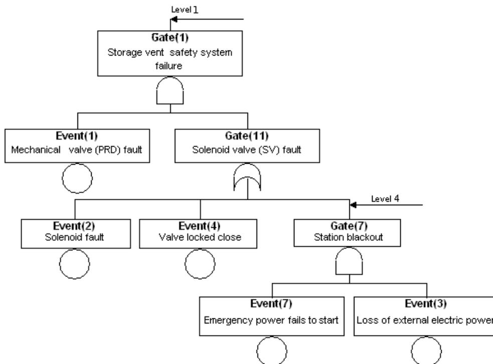
Figure 3. Storage vent emergency system failure sub-fault tree.
