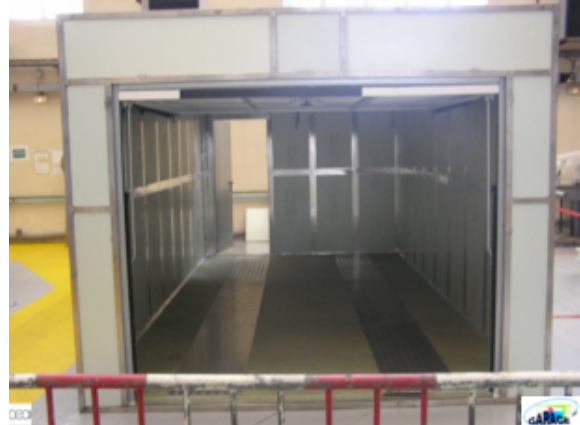
(b) GARAGE structure equipped with Styrodur® sheets
