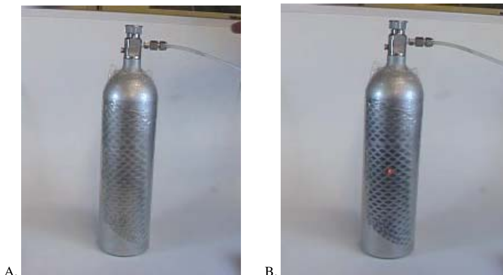
Figure 2. A low-pressure cylinder wrapped with thin film WO 3 :Pd coated indicator "shrink wrap" film. A (before) and B (after) admitting low pressure forming gas to the cylinder. The cylinder has an intentional 57 micron hole near the laser pointer spot on B. Notice the darker indicator pattern in B that developed within a few seconds of pressurizing the cylinder.
