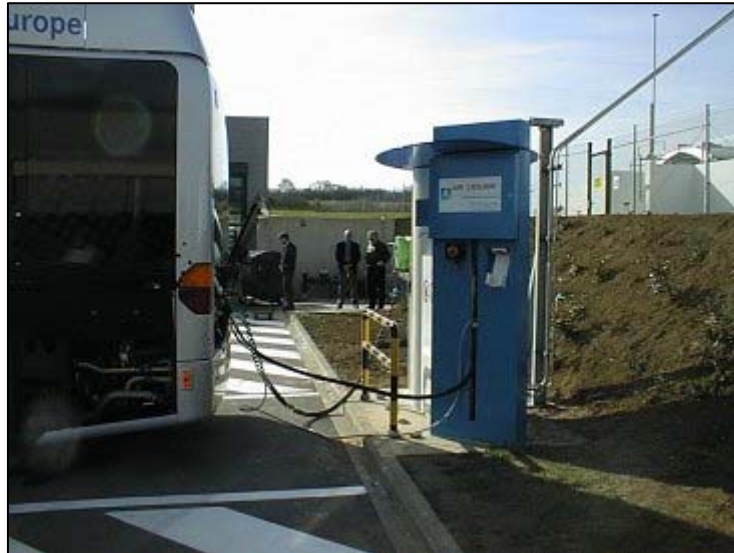
Figure 9: Refuelling of a fuel cell bus in Luxembourg (Photo: Hydro)
