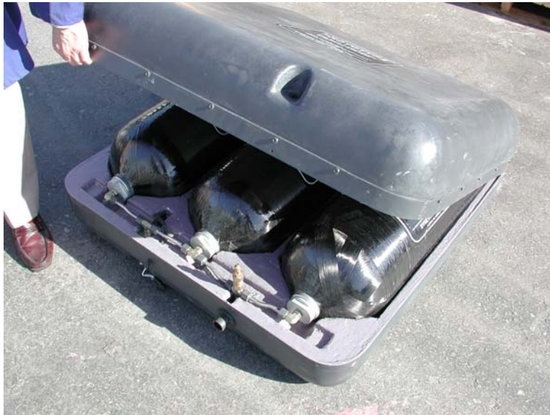
Figure 4: Protective shell encapsulating a fire resistant foam can impart fire protection and an additional level of impact protection to the fuel system.
