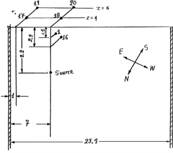
Figure 1 - Sensor and source locations for the BAM experiments (taken from [7])
