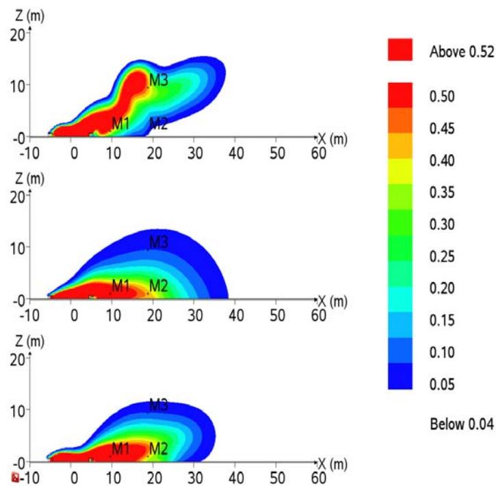
Figure 5 – Volume fraction contours of hydrogen 20s after spill started in the XZ plane at  $Y = 0$  m. [Top] Stable (F) stability. [Middle] Unstable (B) stability. [Bottom] Neutral (D) stability. The annotations M1, M2 & M3 show the positions of the measurement sensors
