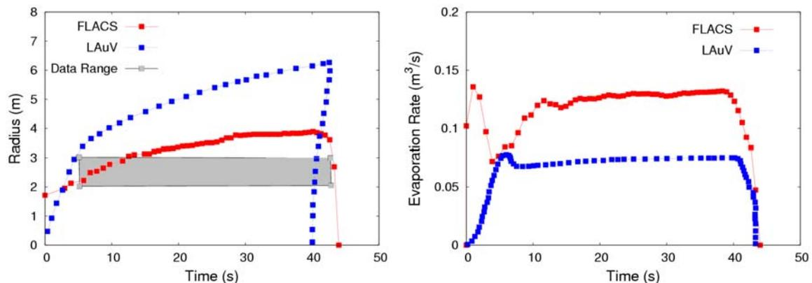
Figure 4 – Comparison of pool spreading and vaporization rate between the FLACS code, the LAuV code and experimental data for NASA Test 6.
