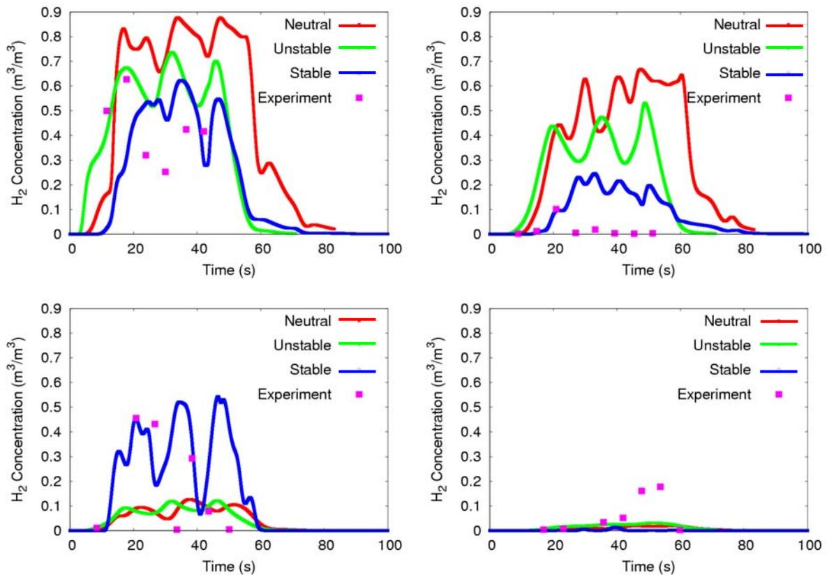
Figure 6 – Time series of hydrogen volume fraction at four different sensors. [Top Left] Tower 2 (height 1 m). [Top Right] Tower 5 (height 1 m). [Bottom Left] Tower 5 (height 9.4 m). [Bottom Right] Tower 7 (height 9.4 m).
