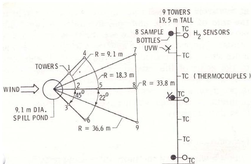
Figure 3 - Deployment of instrumentation towers and typical instrumentation array (taken from [8,9]).
