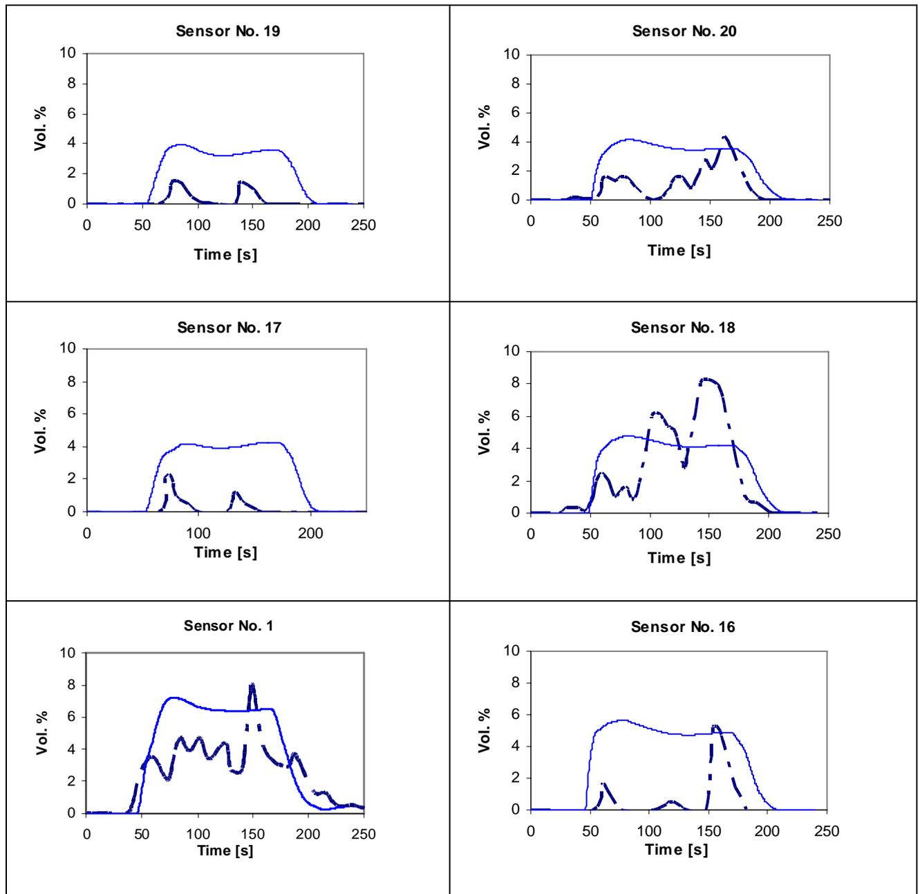
Figure 2 - Comparison of experiments (dotted lines) and simulations (solid lines) for the BAM experiments [7,10]. Top: Sensors 19 and 20, Middle: Sensors 17 and 18, Bottom: Sensors 1 and 16.
