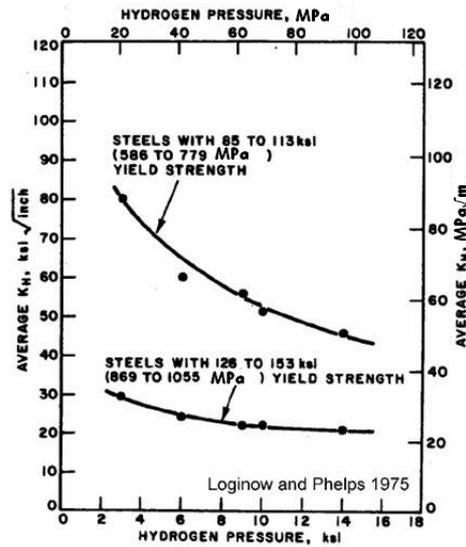
Figure 5: Influence of hydrogen pressure on threshold stress intensity factor at crack arrest [17]
