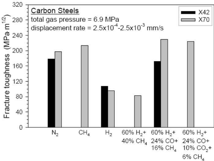
Figure 15. Fracture toughness vs. gas composition for two carbon steels [10]
