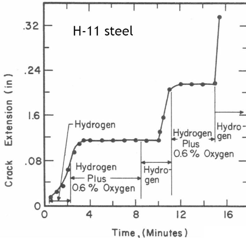
Figure 19. Crack extension vs. Time for hydrogen-oxygen mixtures [7]
