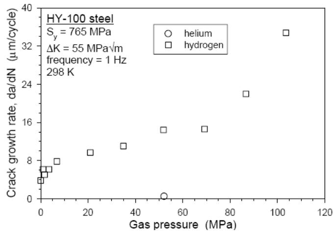
Figure 12. Pressure-dependent FCGR for HY-100 steel [10]
