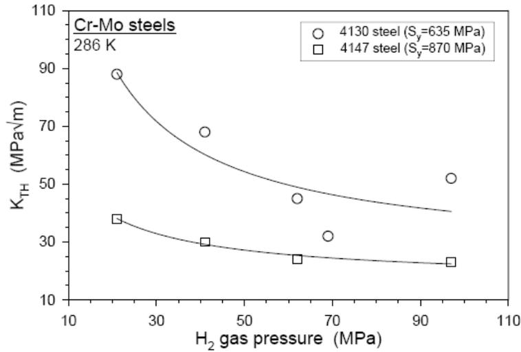
Figure 7. K<sub>TH</sub> for two ferritic steels. HE appears to have little effect on type 4147 at pressures higher than 60 MPa [10]
