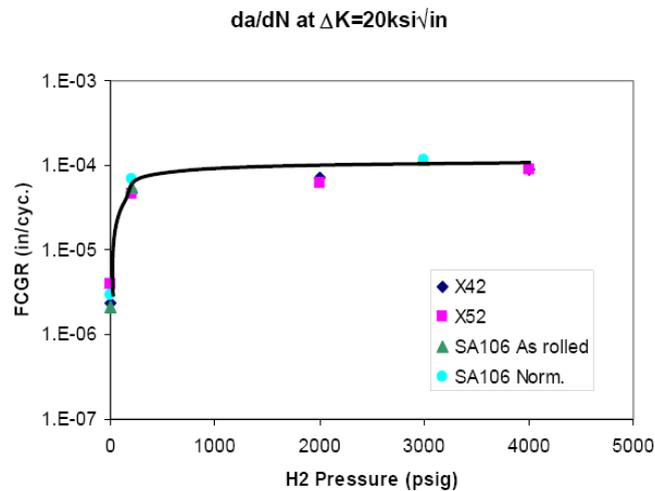
Figure 13: FCGR vs. Pressure for several carbon steels at  $\Delta K=20$  ksi $\sqrt{in}$  [8]
