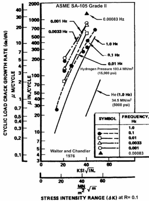
Figure 11. FCGR vs.  $\Delta K$  for SA-105 steel at 103.4 MPa [17]
