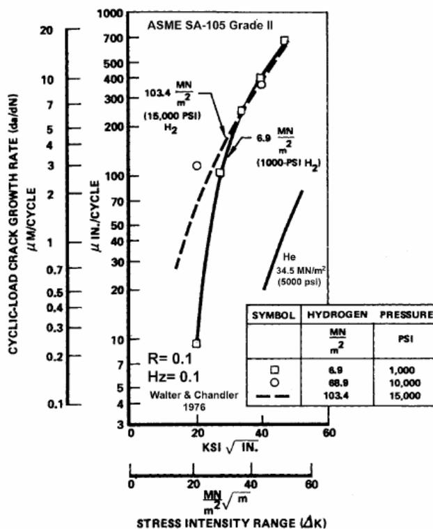
Figure 14. FCGR vs. stress intensity for SA-105 steel at 6.9 and 103.4 MPa [17]
