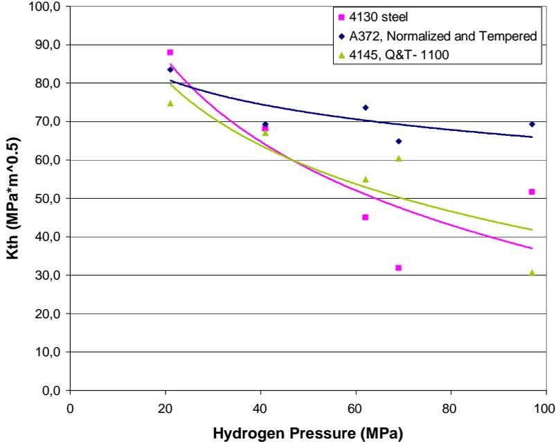
Figure 4. Threshold stress intensity factors for several moderately affected carbon steels [8]
