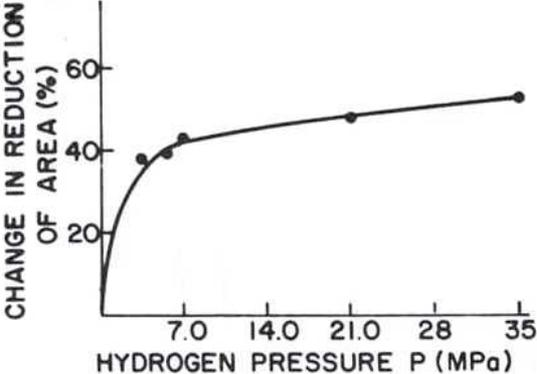
Figure 3. Influence of hydrogen pressure on reduction in area losses for steel similar to X-42 [6]
