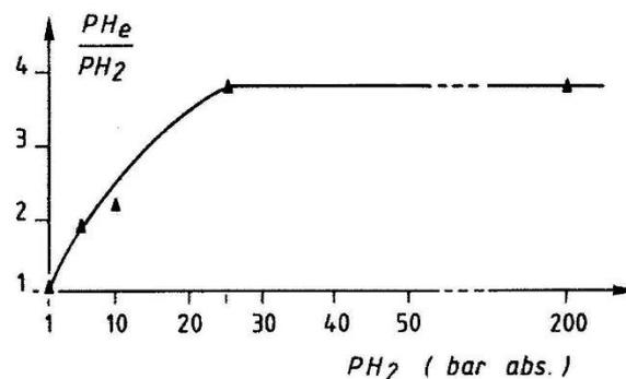
Figure 2. Effect of hydrogen partial pressure on the embrittlement index of AISI 321 steel [2]
