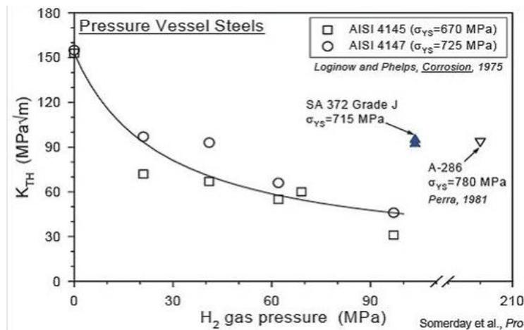
Figure 6. Influence of hydrogen pressure on KTH for several steels [9]
