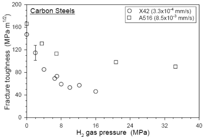
Figure 8: K<sub>IC</sub> for carbon steels. Fracture toughness decreases significantly at low hydrogen pressure before reaching a limiting value [10]
