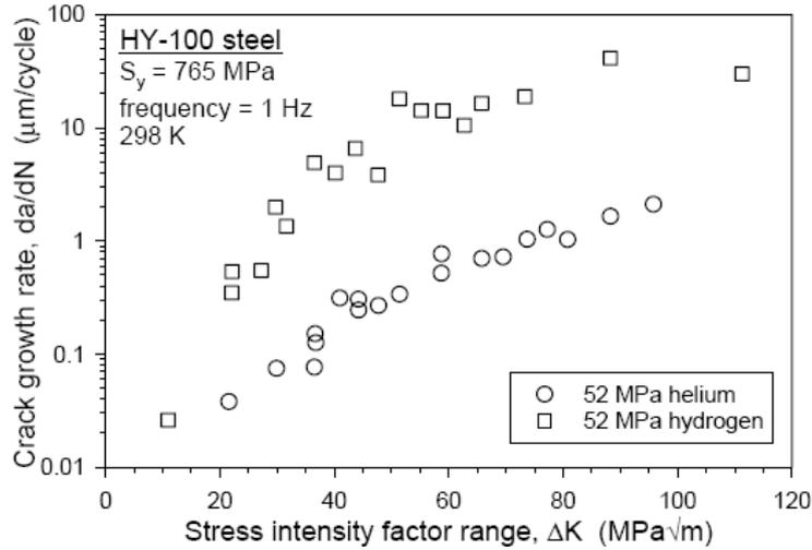
Figure 10. Fatigue crack growth rate vs. stress-intensity factor range for tests of HY-100 steel at 52 MPa [10]
