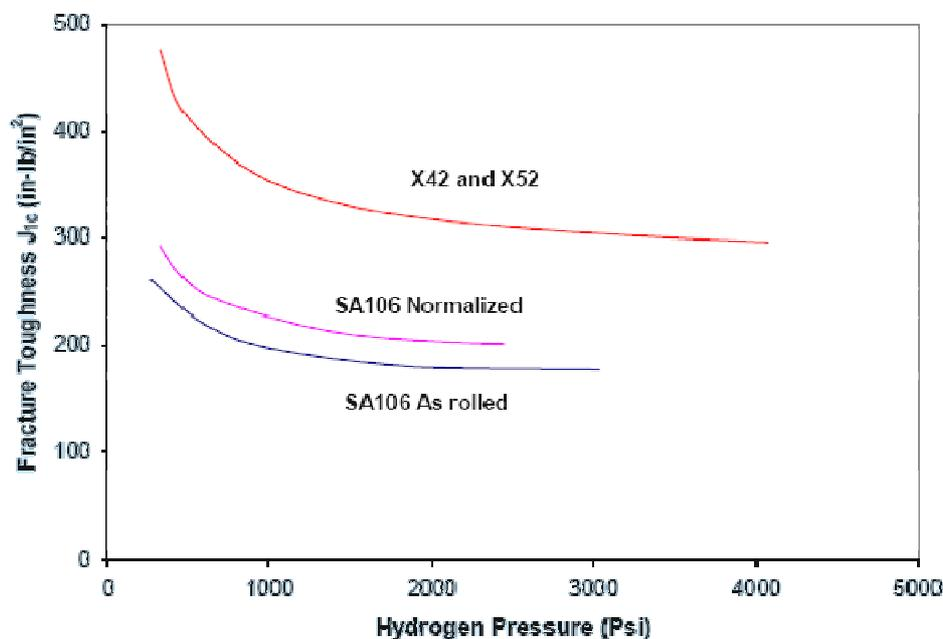
Figure 9. KIC for linepipe steels. Fracture toughness for tests performed at a loading rate of 0.002 in/min [8]
