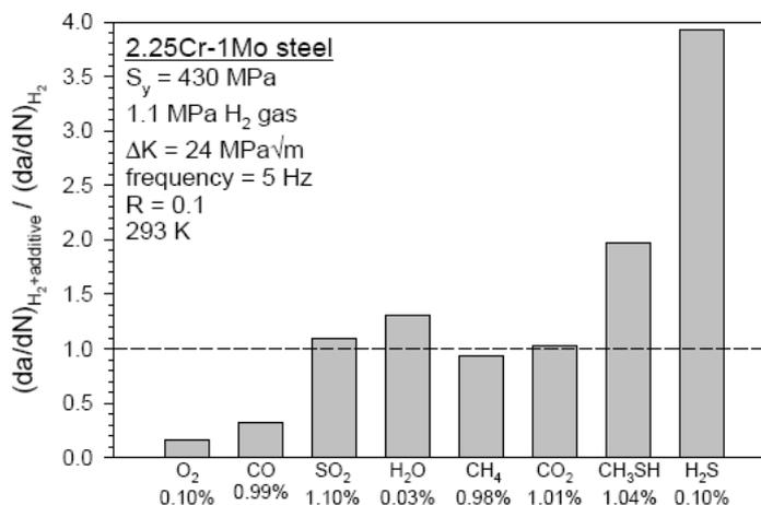
Figure 16: Ratio of FCGR with impurities to FCGR in pure hydrogen at fixed pressure and stress intensity range for a low-alloy ferritic steel [10]
