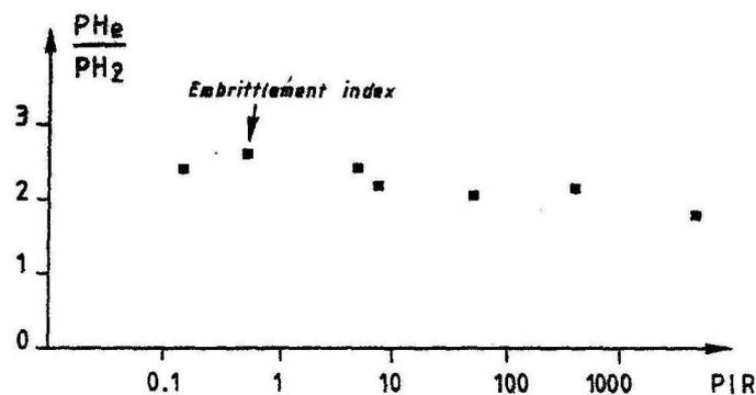
Figure 1. Effect of Pressure Increase Rate (PIR, in bar/min.) on the embrittling index of an unspecified steel during disk rupture testing [2]
