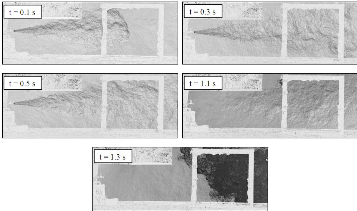
Figure 7. Sequence of BOS-photos of experiment #64 ( $M_{H_2}=203$  g,  $W_{aver}=188$  g/s).
