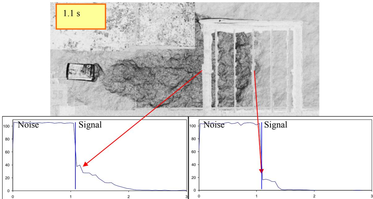
Figure 16. BOS photo after end of injection and concentration gauges records, experiment #55
