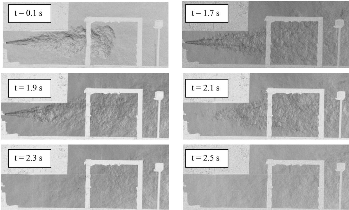
Figure 6. Sequence of BOS-photos of experiment #65 ( $M_{H_2}=402$  g,  $W_{aver}=193$  g/s).
