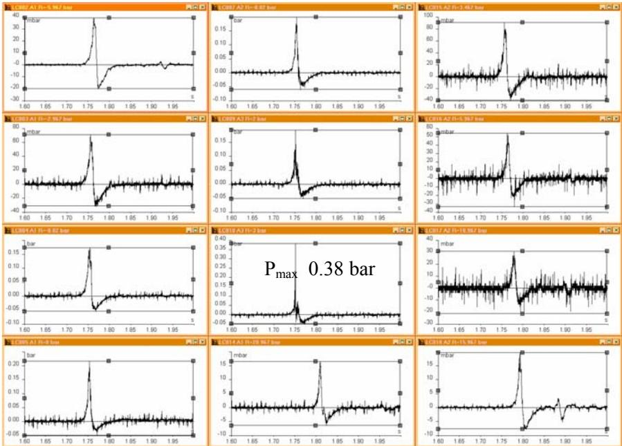
Figure 9. Pressure records of all gauges, experiment #58
