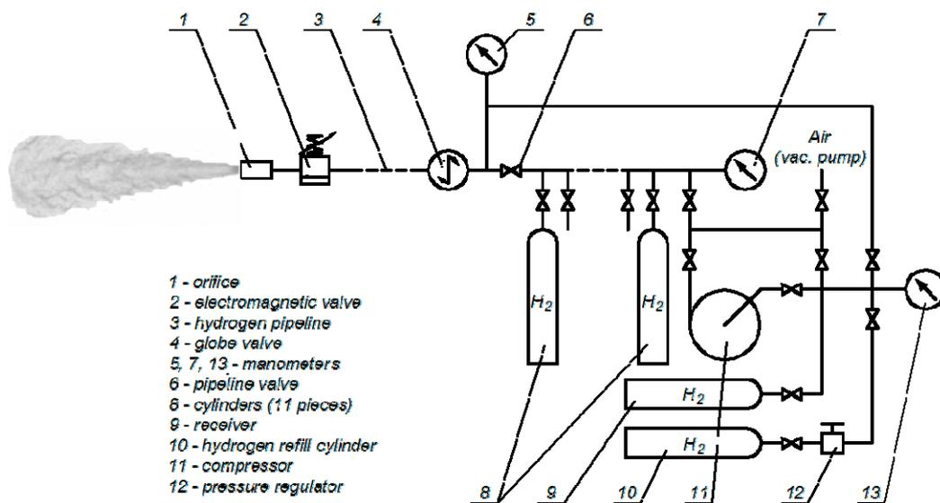
Figure 3. System of hydrogen supply.
