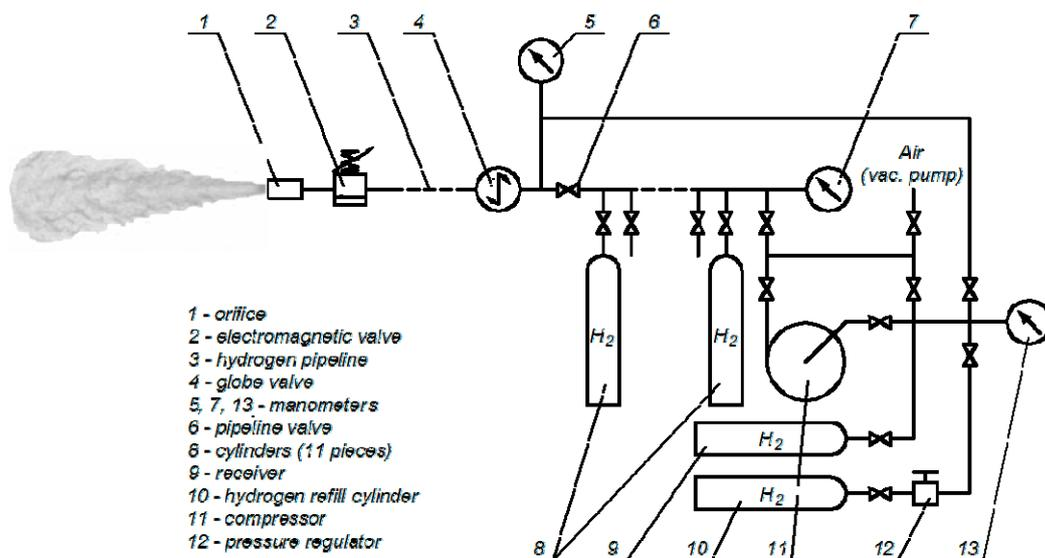
Figure 3. System of hydrogen supply.
