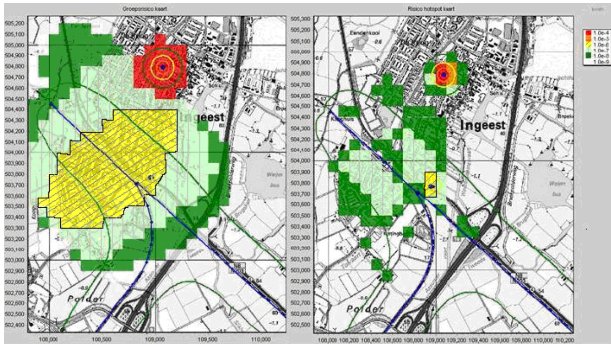
Figure 2a and b. Representation of societal risk as developed by TNO and RIVM in the Netherlands, not as the usual F , -N curve of all possible scenarios a risk source or cluster of sources can produce ( F = Frequency of exceedance of N fatalities versus the number N ), but as a location-specific value in a 50 \times 50 \text{ m}^2 area indicated by color (or here grayscale). Population density data are embedded in each cell. A F , -N curve is calculated for each cell taking into account only risk sources that affect the cell but fatalities due to it in the whole area, left , and right of only the fatalities in the 50 \text{ m}^2 square cell. Subsequently, the position of the F , -N curve versus the norm is translated into color e.g. figure left : (red) – dark area middle top with dot - = above the norm; orange - not present - a factor 10 below, yellow – outlined diagonally dashed area center left – a factor 100 below, light green – periphery lightly vertically dashed - safe, and green – periphery dark - very safe). The right figure serves to find more easily the hazard ‘hot spots’. This example concerns a railway shift yard and a stationary risk source [24]. The small circles represent risk contours around a static risk source.
