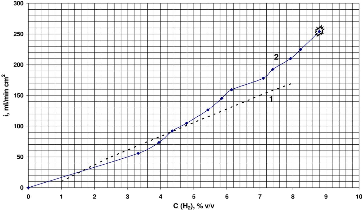
Figure 2. Specific recombination reaction rates vs. concentration of hydrogen for PAR model FR/1-90 (Siemens) (1) and for HCm cartridge (2).
