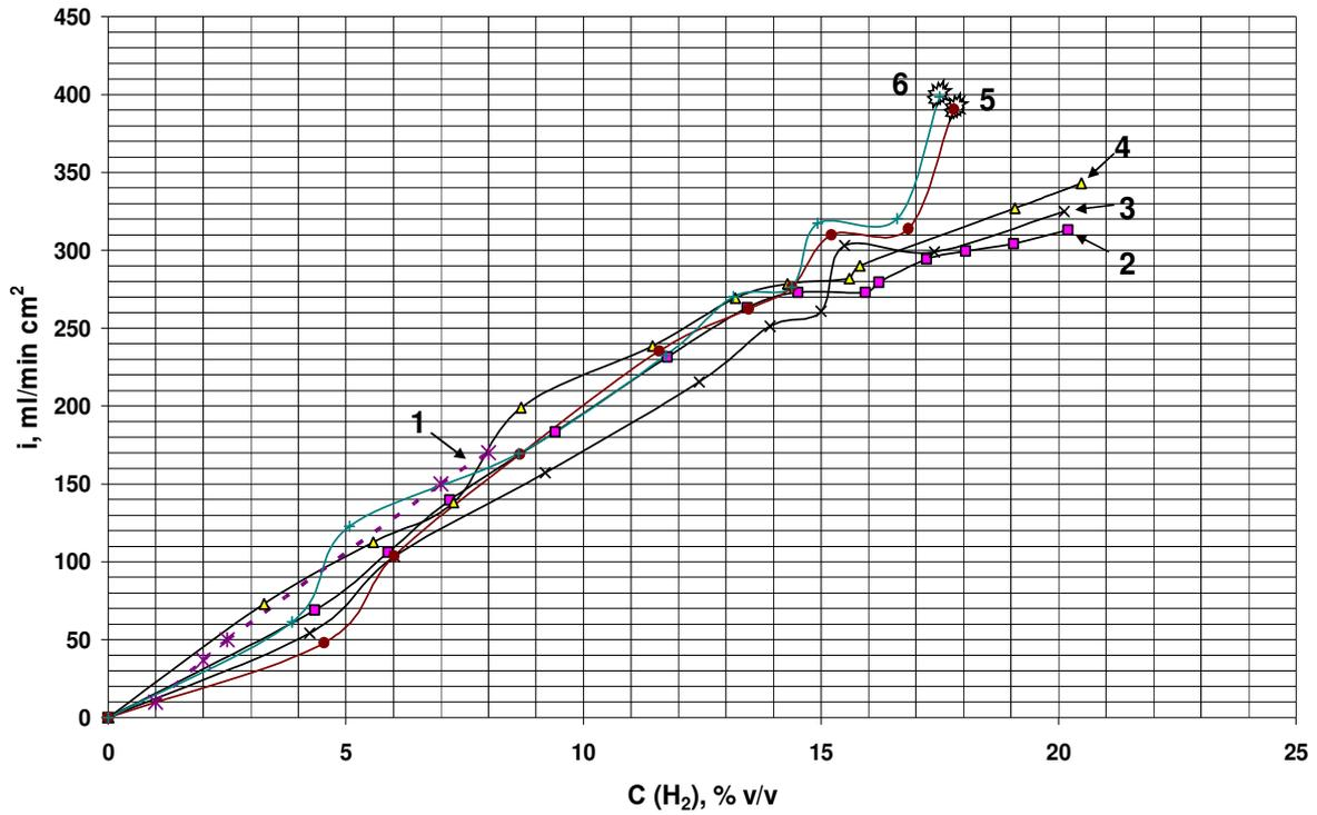
Figure 4.  $i$ - $C$  graph for recombination reaction at stationary conditions for FR/1-90 model [6] (dash line 1) and for experiments with 4-plate cartridges of HCm(screen) catalyst (2 - 6).
