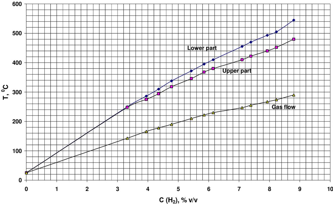
Figure 3. T-C graph for the lower and upper parts of HCm plate and for gas flow above the cartridge.
