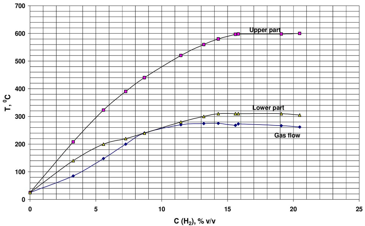
Figure 5.  $T$ - $C$  graph for the lower and upper parts of HCm(screen) catalyst plate and for gas flow above the cartridge.
