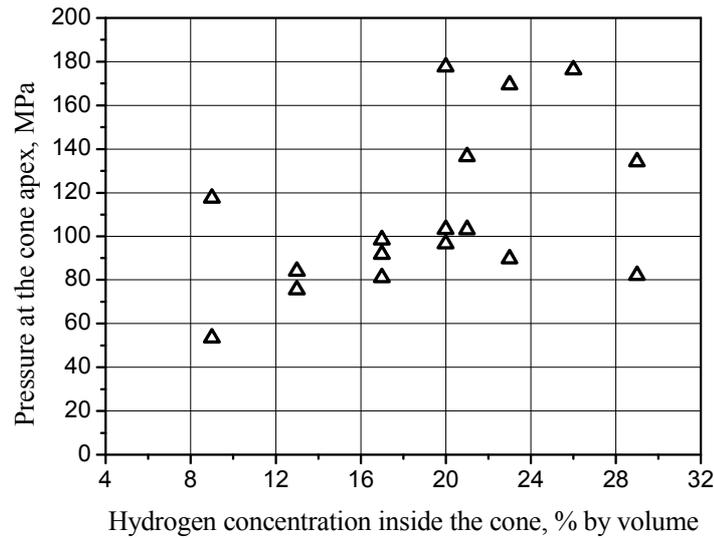
Figure 4. The experimentally obtained pressures in the cone apex for the first series of experiments. The rubber envelope contained a stoichiometric hydrogen-air mixture.
