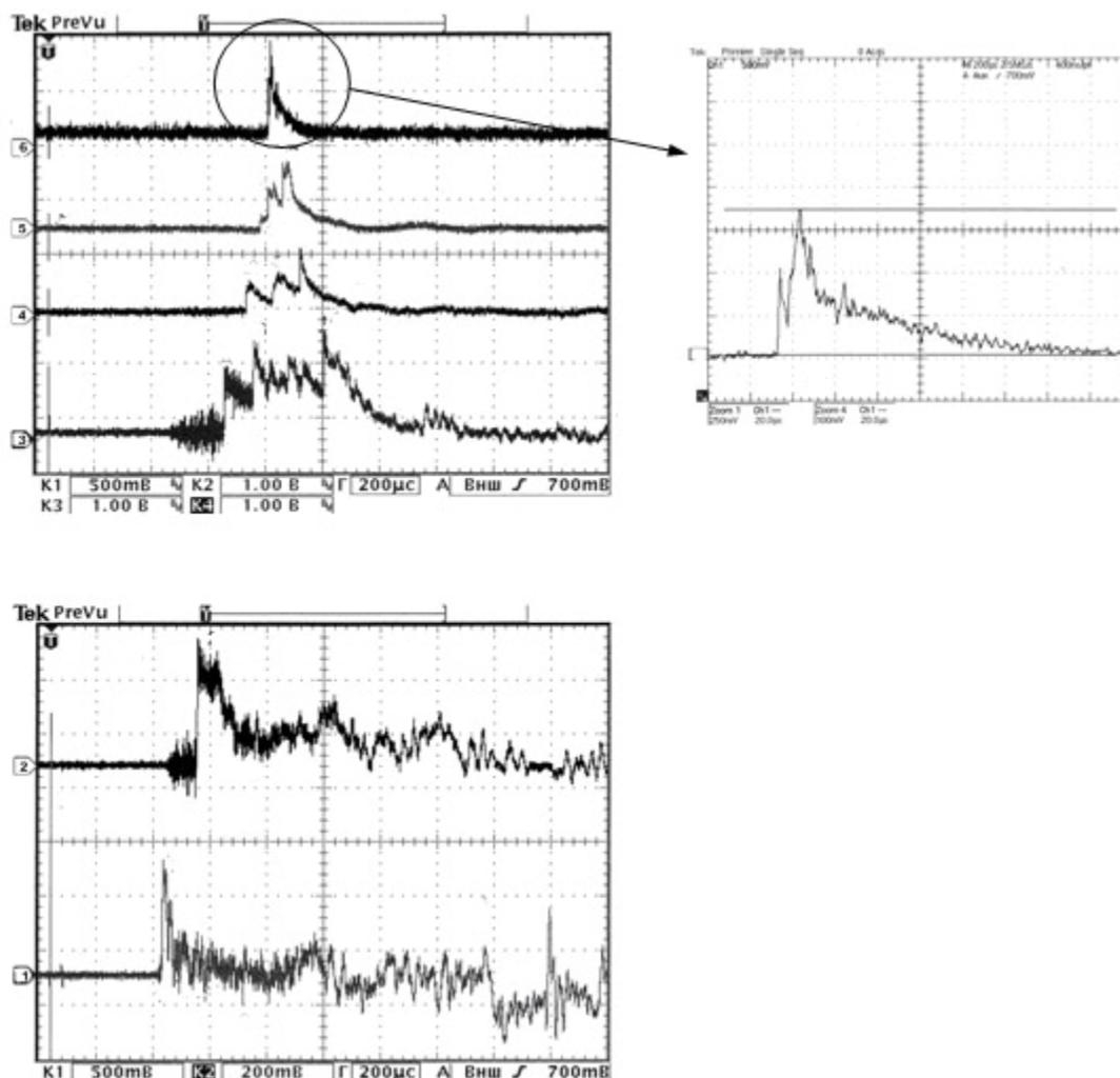
Figure 3. Oscillograms of pressure sensor signals. Two-chamber mode, in the cone –17%  $\text{H}_2$ +air; in the rubber envelope – stoichiometric mixture. At upper right –oscillogram of signal of sensor 6 with increased time resolution.
