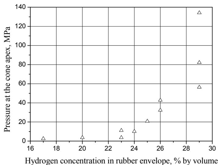
Figure 5. Maximum pressure as a function of H<sub>2</sub> concentration in the rubber envelope. Concentration of H<sub>2</sub> in the cone is equal 29% by volume. Initiation was made by blasting 0.8 g of PETN.
