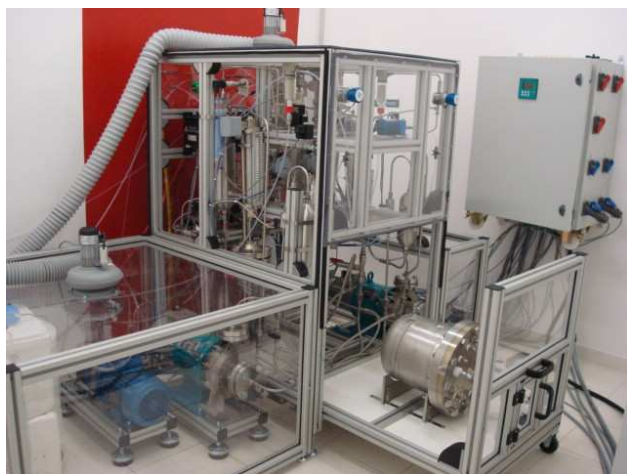
Figure 8. General view of the GenHy ® 1000 high pressure water electrolyzer on the test bench, in the test room.
