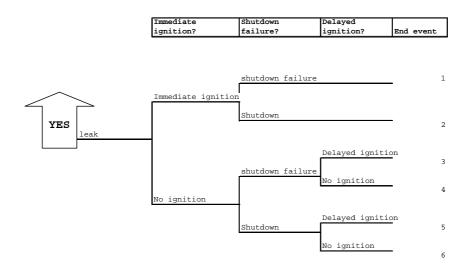
Figure 2. Illustration of the event tree used for the dispensers in the QRA
