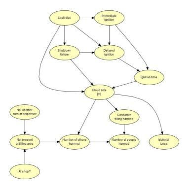
Figure 6. Bayesian network modelling of the dispenser area of the hydrogen refilling station. The top four nodes are equivalent to the original event tree
