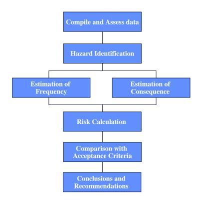
Figure 1. Illustration of the QRA process
