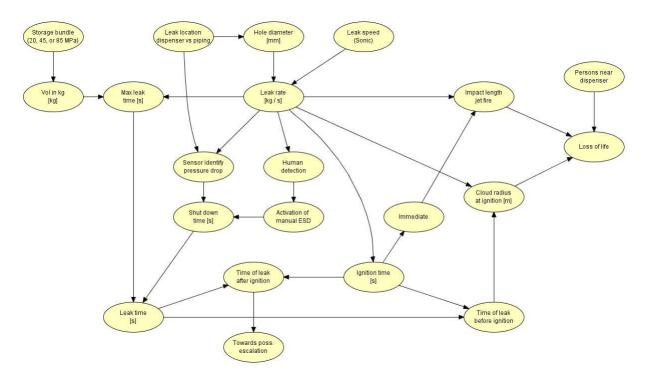
Figure 7. Extended Bayesian network modelling of the dispenser area of the hydrogen refuelling station
