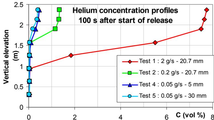
Figure 2: Vertical helium concentration profile in the garage for tests 1, 2, 4 and 5; 100 s after the start of the release
