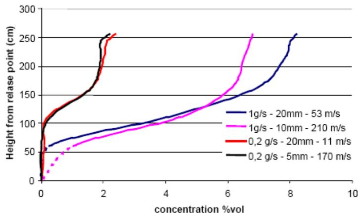
Figure 1: Vertical concentration profile at end of release for various release rates, according to Lacomme et al. (2007)
