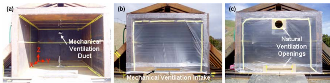
Figure 1. Garage facility with mechanical (a and b) and natural (c) ventilation configurations.
