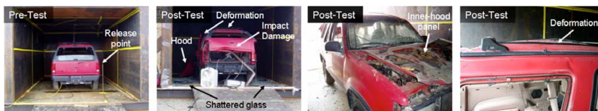
Figure 6. Pre-test and post-test photos of damage to the vehicle caused by an internal hydrogen-air deflagration.
