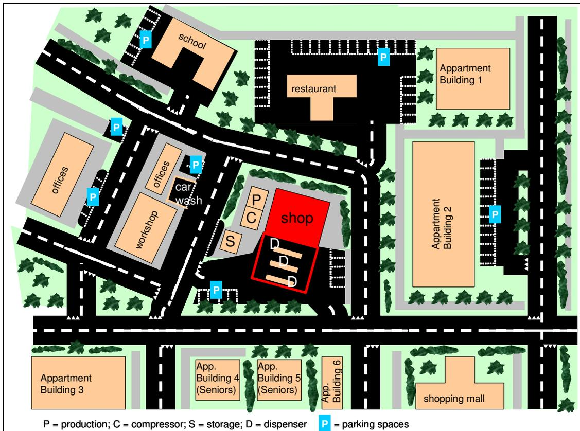
Figure 2. Layout of BBC refuelling station and its surroundings
