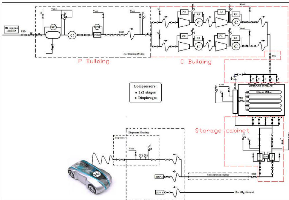
Figure 1. Simplified process scheme of the BBC refuelling station
