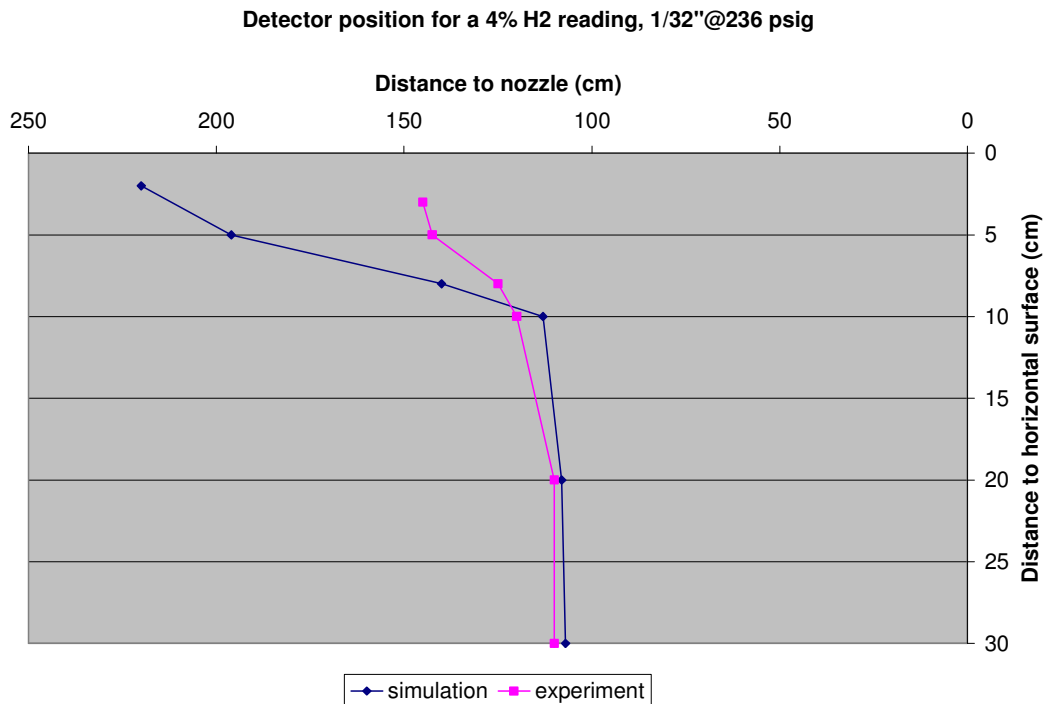
Figure 3 – Effect of the nearby ground (horizontal surface) on the length of the LFL cloud
