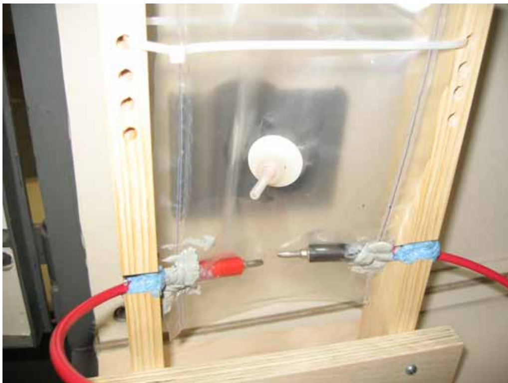
Figure 3 – Setup used to ignite hydrogen inside a bag using a calibrated electrostatic discharge device.
