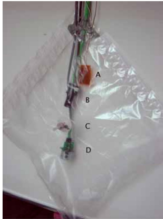
Figure 1 – Instrumented Hydrogen bag: A) thermal flux sensor, B) spark plug, C) hydrogen valve, D) Hydrogen detector
