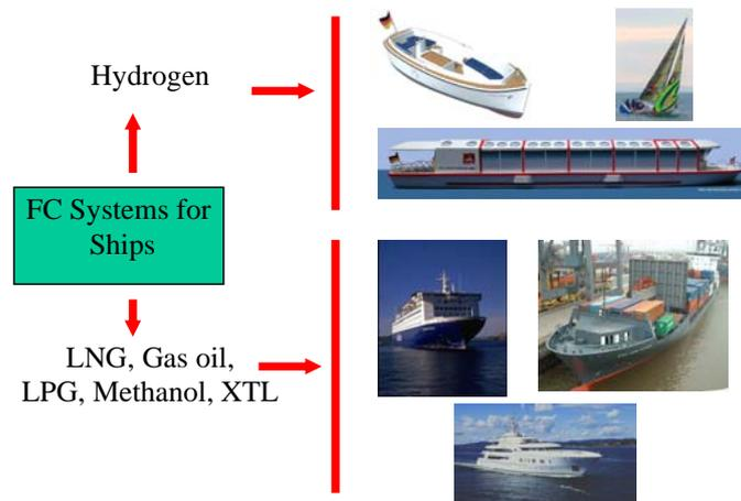
Figure 2. Which fuel for which application?
