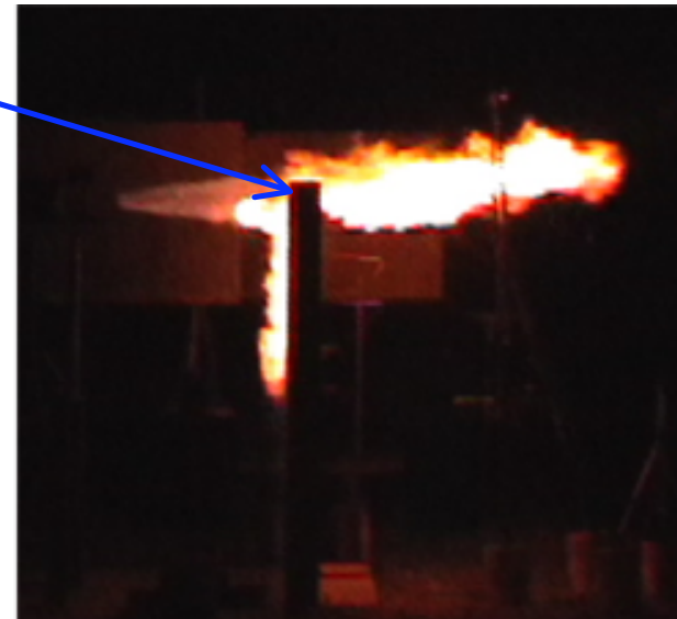
Jet Centered on Top of 1-Wall Barrier
