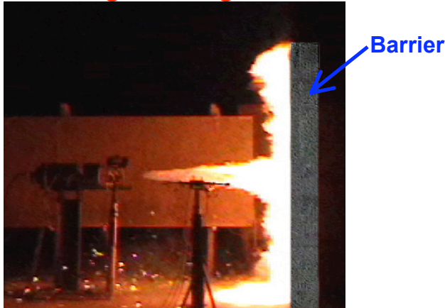
Sandia/SRI H 2 Jet Flame Barrier Test
