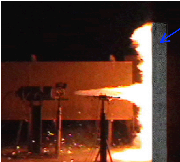
Jet Centered on 1-Wall Barrier
