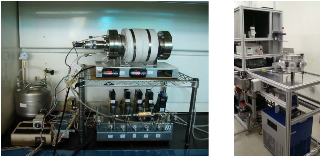
Figure 2: Hydrogen safety sensor test apparatus. (Left) Apparatus designed and built at the Illinois Institute of Technology currently deployed at NREL. (Right) New sensor test apparatus under construction at NREL with enhanced performance capabilities
