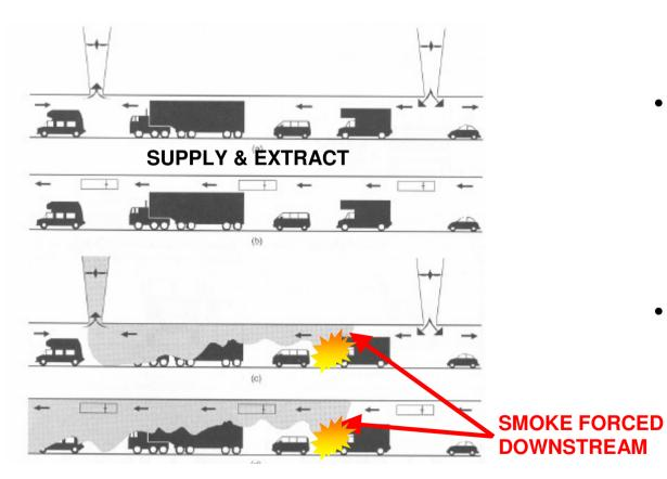
In normal operation ventilation removes emissions and provides fresh air
