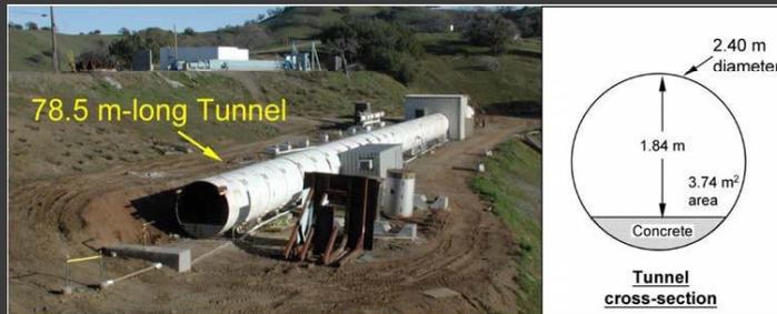
1/5 real-scale experiments on hydrogen-air deflagration in tunnel
