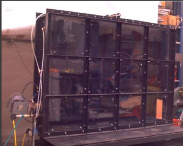
The experimental rig 1.20 m × 0.20 m × 0.90 m, with compartments 0.30 m × 0.20 m
