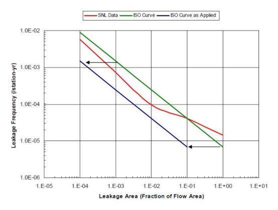
Figure 2 Comparison of valve leak frequency distribution used in NFPA and ISO analyses [5].
