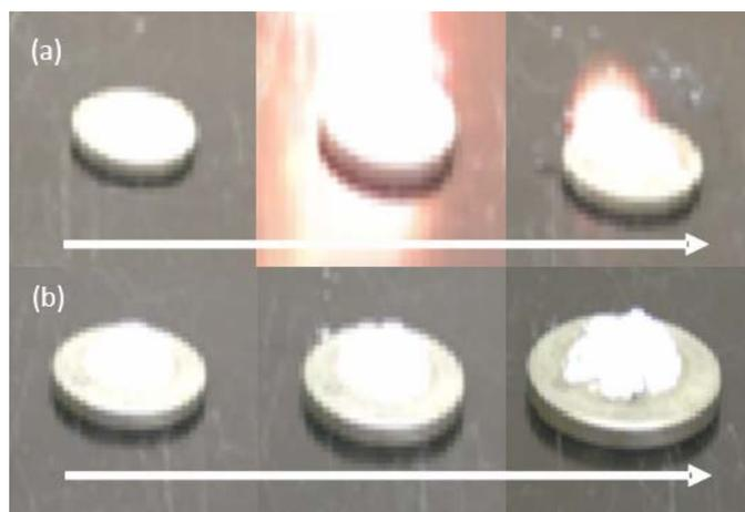
Figure 5. Water Drop Test of (a)  $\text{LiBH}_4$ , and (b) 5 mol %  $\text{LiOH-LiBH}_4$ .
