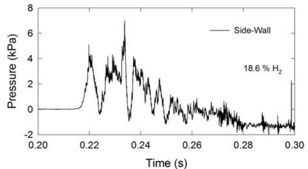
Figure 11. Differential pressure traces recorded over two times during an experiment in which an 18.6 % hydrogen/air mixture was ignited with a vehicle present.
