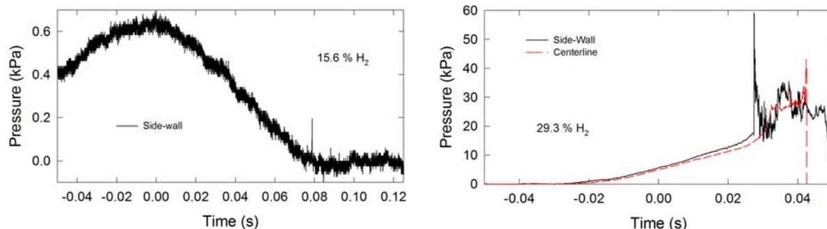
Figure 7. Overpressure time histories for experiments without a vehicle and ignition with indicated hydrogen concentrations at the ignition location.
