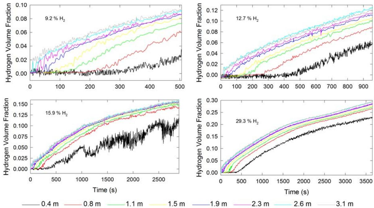
Figure 2. Examples of hydrogen volume fraction temporal profiles measured in garage without a vehicle during the period between hydrogen flow initiation and hydrogen/air mixture ignition.
