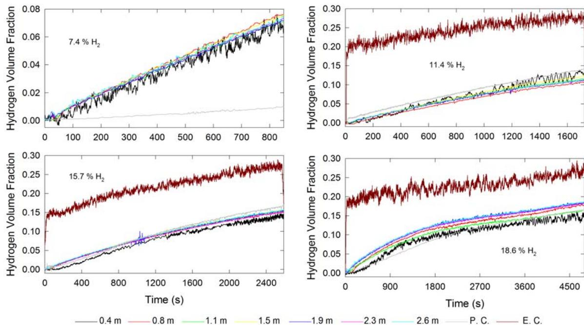
Figure 3. Examples of hydrogen volume fraction temporal profiles measured in garage with vehicles during the period between hydrogen flow initiation and hydrogen/air mixture ignition.
