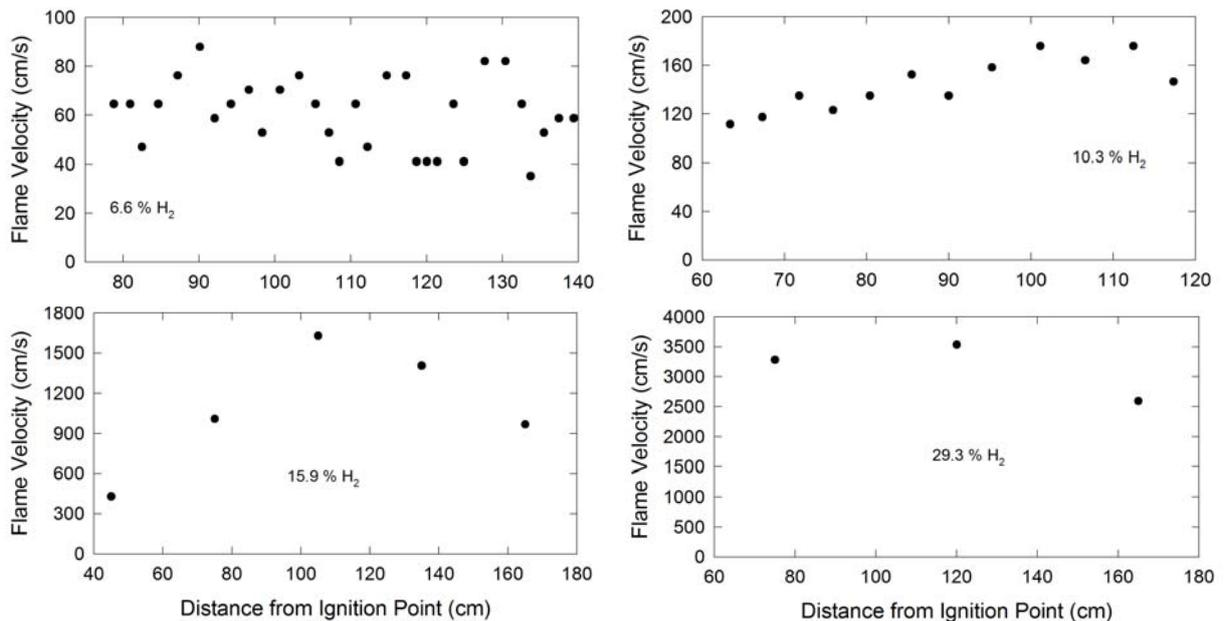
Figure 5. Flame spread velocities measured following ignition of hydrogen/air mixtures having indicated volume fractions at the ignition location.
