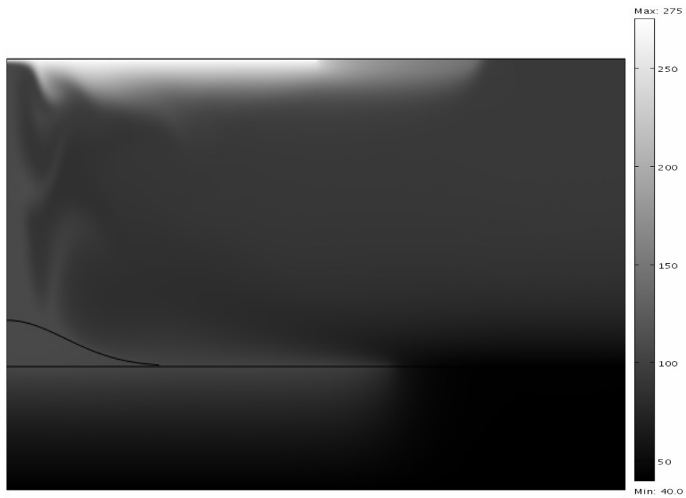
Figure 10 – Temperature plot (°C) during first dehydrogenation reaction of AB.
