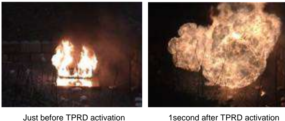
Figure 1. a HFCV fire test is caused by a gasoline pool fire
