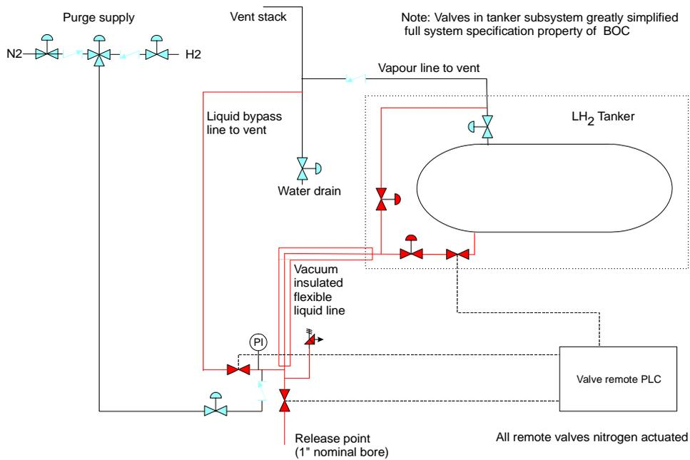
Figure 1. Schematic of release system
