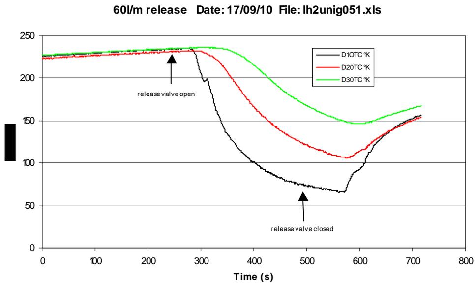
Figure 7. Concrete temperatures during the release
