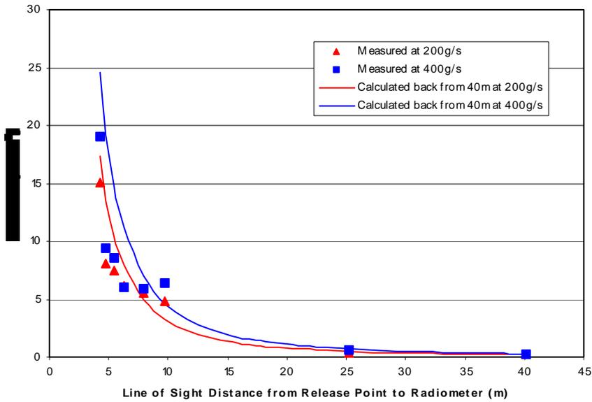
Figure 9. Measured heat flux intensity versus inverse square law calculation – 2” Pipe
