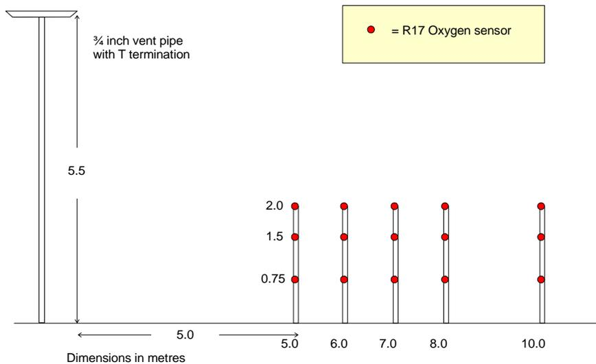
Figure 7. Location of oxygen sensors relative to release point
