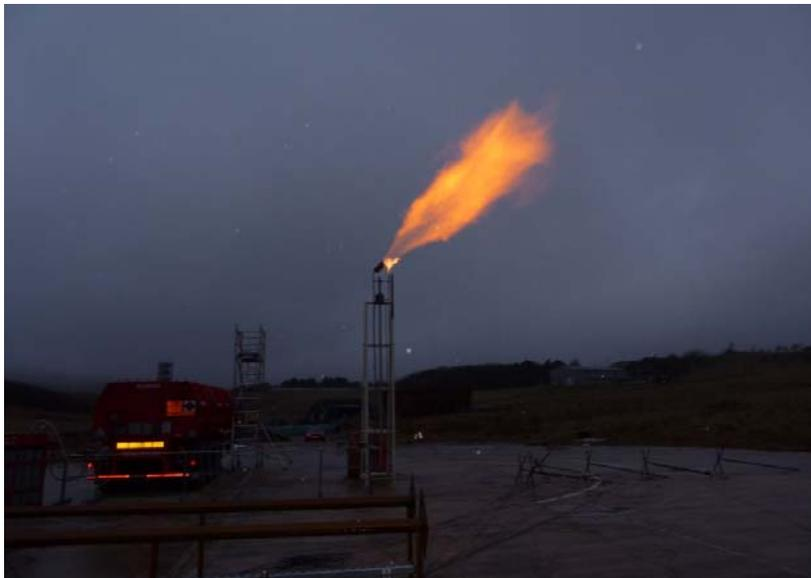
Figure 6. Visible flame releases – 45° shrouded vent termination
