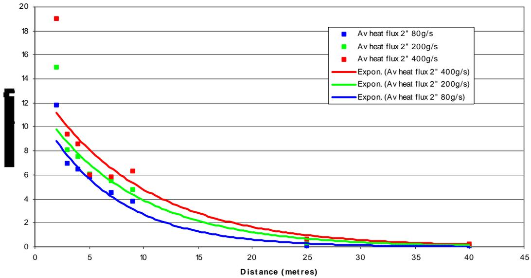
Figure 11. Heat flux intensity against distance – 2" Pipe
