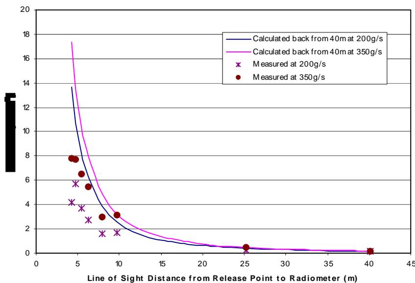
Figure 8. Measured heat flux intensity versus inverse square law calculation – 3/4" Pipe
