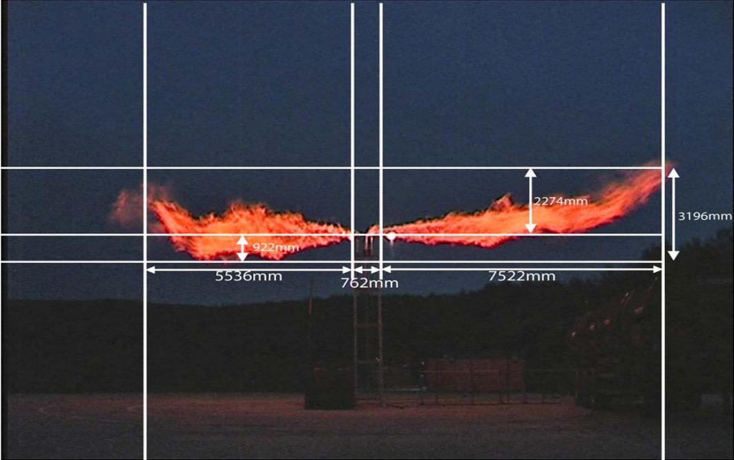
Figure 4. Visible flame releases – 2" Pipe 400g/s release T-piece fitted
