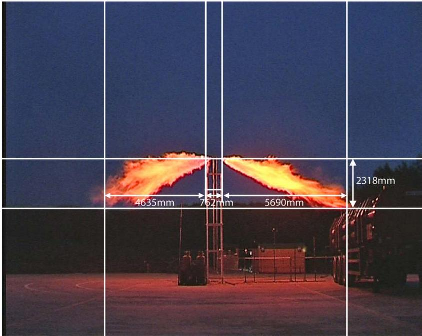
Figure 5. Visible flame releases – 3/4” Pipe 350g/s release T-piece fitted
