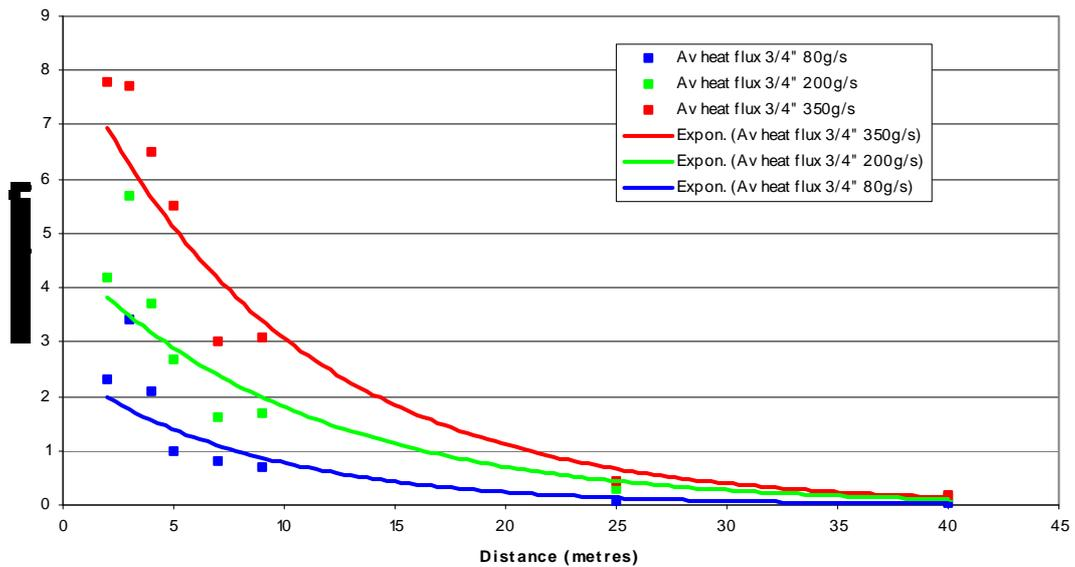
Figure 10. Heat flux intensity against distance – ¾” Pipe
