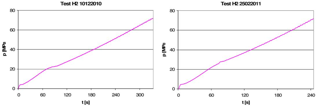
Figure 2. Hydrogen pressure profiles at tank inlet.
