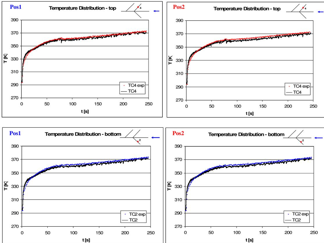
Figure 9. Predicted temperature inside the tank at thermocouples position, compared with experimental data (Test H2 25022011).
