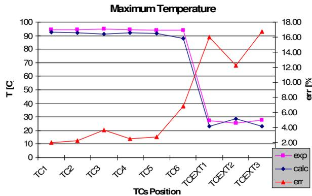
Figure 7. Accuracy of predicted maximum temperature at TCs position (Test H2 10122010).
