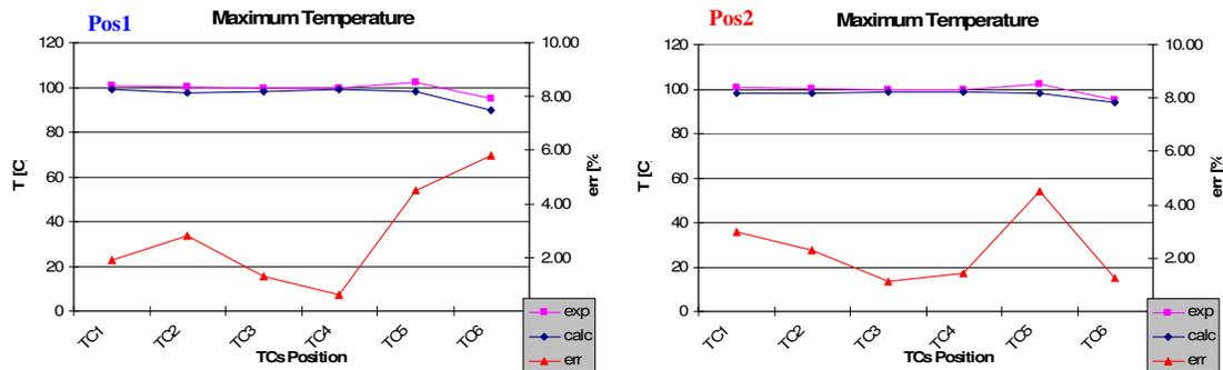
Figure 10. Accuracy of predicted maximum temperature at TCs position for Pos1 and Pos2 (Test H2 25022011).
