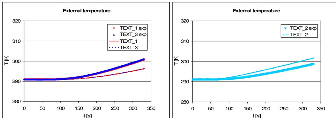
Figure 6. Predicted temperature outside the tank (left) and on the inlet boss (right) at TCs position, in comparison with experimental data (Test H2 10122010).
