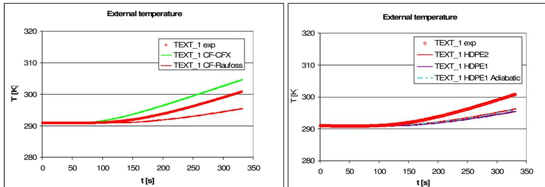
Figure 8. Sensitivity to material properties (left) and external heat transfer BC (right) (Test H2 10122010).
