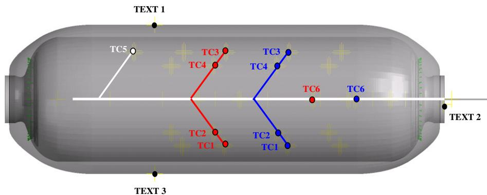
Figure 1. Thermocouples (TCs) position inside and outside the tank: Pos1 (blue), Pos2 (red), fixed internal (white) and external (black) ones.
