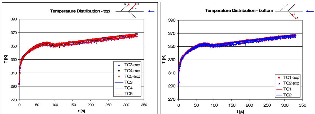
Figure 5. Predicted temperature inside the tank at thermocouples position, compared with experimental data (Test H2 10122010).
