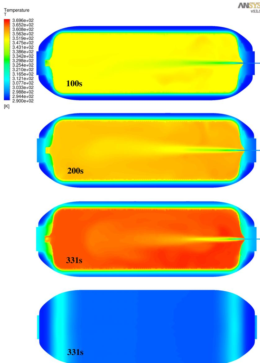
Figure 4. Temperature contours plot at different time interval from the start of the filling, inside and outside the tank (figure at the bottom) (Test H2 10122010).
