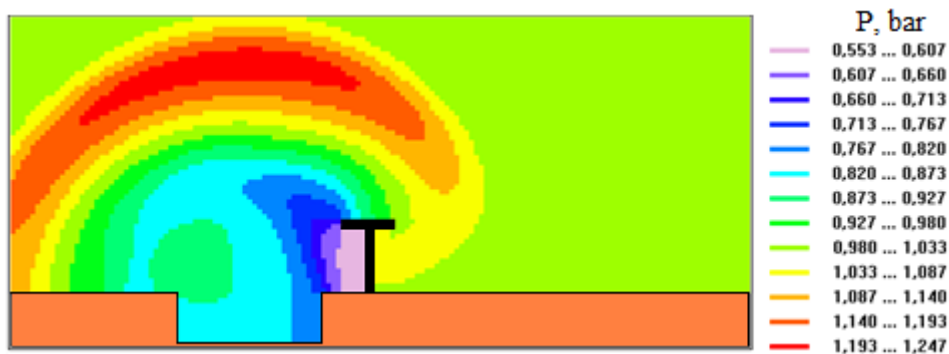
Fig. 20. Pressure distribution at the moment 0.023 \mu s after the explosion (case 10)
