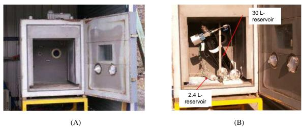
Figure 5. Pictures of the INERIS experimental installation. (A) climatic enclosure, (B) climatic enclosure with device for tests.
