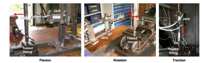
Figure 6. Pictures of the different configurations of the "dynamic stress" module.
