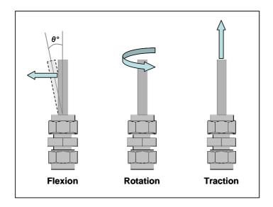
Figure 3. Scheme of "dynamic stresses" applied on 6 mm double ring tube fittings.
