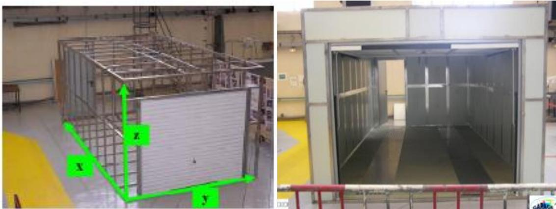
Figure 1. Description of GARAGE set-up at CEA Saclay (a) Left: structural steel skeleton and (b) Right: interior of the facility with the panels
