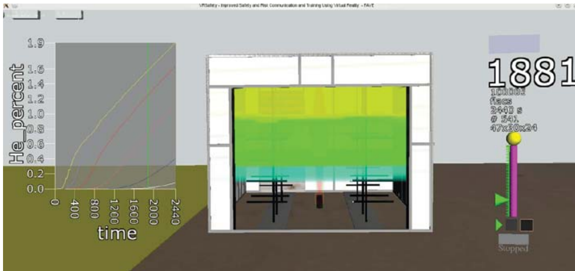
Figure 3 VRSafety visualization of dispersion simulation (CEA Garage test 5, 0.05 g/s He injected into a garage sized enclosure). The gas is released centrally on the floor (see red plume from black cylinder) and the different colours show gas concentrations. To the right the progress bar can be seen, illustrating that this is a FLACS simulation 1881s after start of the release. To the left gas concentrations at 6 sensors can be seen, the green vertical line shows the current time in the animation.
