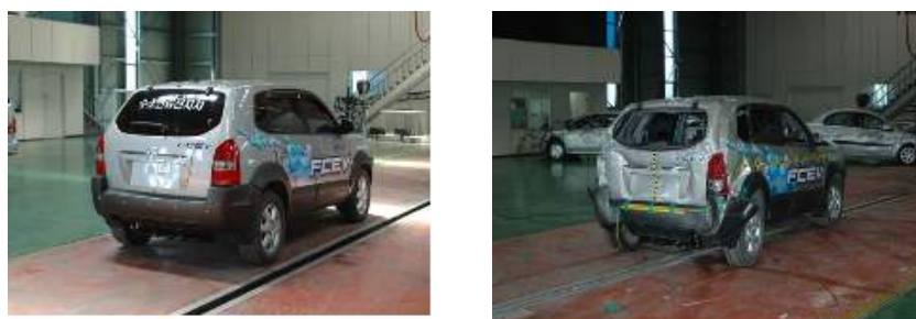
Figure 5. Rear-right view of the test vehicle before and after test.
