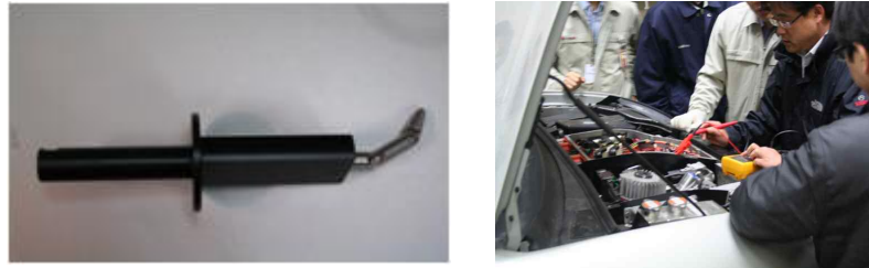
Figure 15. IPXX B (test wire) and bonnet evaluation.
