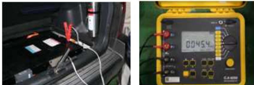
Figure 18. The supercapacitor enclosure and the chassis evaluation.
