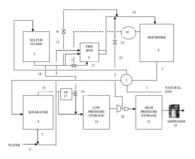
Figure 1: Schematic of H-CNG Process
